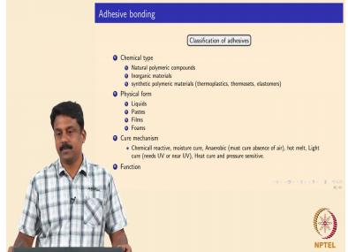
So how do you classify the adhesives? We can classify in various ways. So chemical type or physical forms or cure mechanism, how you cure that or a function. Right? So the chemical types, so now it can be natural polymeric components, okay inorganic materials, or synthetic polymers like thermoplastic, thermosetting, the elastomers. Nowadays we have all the high-temperature glues. Even those are all thermoplastic. Okay.
