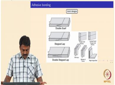
Some of the joint designs I gave. These are also commonly used for automotive applications. Double scarf, stepped lap, double stepped lap, tongue and groove and ya, right angle butt, you can just refer it from the slides.
