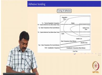
So in in all these processes, curing is achieved by heating above or by curing above the glass transition temperatures. Okay. So for example, this is the curing time and this is the characteristic of the various reactions that is possible in adhesive. Okay. For example crystalline and becoming glass transition and then you have melting. Okay. So generally, the curing is done above melting and then below the degradation temperature. Okay. So this is the optimum cure zone. Okay.
