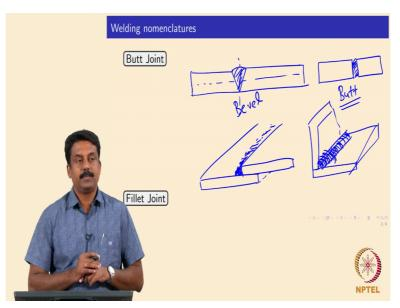
So when you call it is a butt joint, so butt joint when you are joining the 2 flat surfaces or you have joined where the plate thickness is exactly perpendicular to the weld centreline ok. So for example, you make a butt joint so this is butt joint with regroove is not it? So the butt
