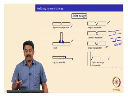
So what are the joint designs? So one thing I showed you already the butt joint right. This is square butt preparation, and butt joints we also have Bevels like single V where you make a single V with an angle ok. And single V is generally done with somewhere lesser thicknesses, but if the thickness of the plate goes higher and we can also go for double V, so why you need double V because we can fill it both sides right, so double V or K is also commonly used, so what is K?
