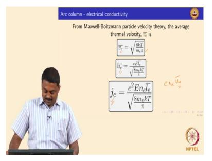
So once we know the drift velocity and we also know that the thermal velocity is square root of 8 k T by m e pi that is the average thermal velocity, so now we have the predictable means of the expressions, ok so we already converted all the variables into the predictable variables. So now if we can replace the (the drif) thermal velocity into this square root of 8 k T by m e pi then we have the expression for the average drift velocity.
