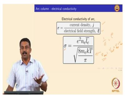
So once we know the expression now the conductivities, current density, the total current density where we can even still keep j e plus j i but again j i is negligible we can take it out, by the field strength E, so that is what conductivity of an arc, ok. So if there is a case the electrical conductivity of an arc, so we give the expression for j E, the E goes out in j E and this is expression to calculate the electrical conductivity of an arc and 1 by sigma is.
