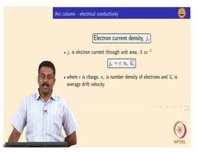
So electron current is nothing but e times the number density and then drift velocity, number density can be calculated from saha equation, ok that gives the amount number of electrons percent is not it, as a function of temperature and drift velocity we even do not know, so we will have to derive many an expression for drift velocity, ok.
