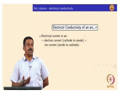
So we will just quickly look at the derivation again, so electrical conductivity of an arc, how do you derive that sigma? So electrical current is we can assume that it is a total current, the electron current plus the ionic current, electron would travel from cathode to anode and ion would travel from anode to cathode. So now we are deriving the equation for the electron current and the ion current.
