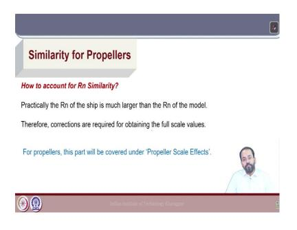
Now, we can maintain Froude number similarity between model and full scale, but we see that the Reynolds number similarity cannot be maintained. It is not feasible because of very high values of velocity and rpm in the model scale if we try to go for Reynolds number similarity.
