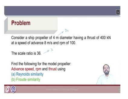
Now, we will do a simple problem based on the model and full scale values of propeller velocities and forces, and how we can use these Froude number and Reynolds number similarity to calculate the values.
