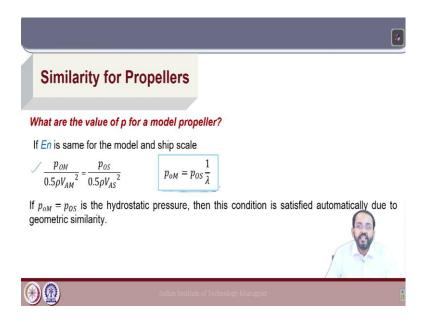
On the other hand, if we look towards the pressure component, if we keep Euler number E p or the pressure coefficient here, same between the model and full scale, we get that the pressure in the model scale is the full scale pressure divided by  $\lambda$ .
