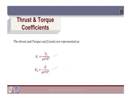
So, the thrust and torque coefficients of the propeller after doing this dimensional analysis can be written in this particular form. In the propeller open water characteristics, this is the primary form of expressing the propeller thrust and torque in non-dimensional form, using  $K_T$  and  $K_Q$  which are the thrust and torque coefficients.
