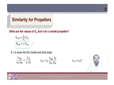
If we do that and assume that the viscosity is same in the model and full scale, we will get the ratio  $V_A$  in the model and full scale as a ratio of the diameters in an inverse way. The model scale propellers advance speed will be  $\lambda$  times the advance speed in the full scale, where  $\lambda$  is the ratio of the full scale diameter by the model scale propellant diameter.
