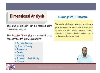
For marine propellers, it is of importance to relate the model scale characteristics to the full scale with the use of certain dimensionless parameters, where we use the laws of similarity to do a dimensional analysis. So, we will use Buckingham  $\Pi$  theorem here, which is a popular theorem used in engineering as well as mechanics problems to relate a parameter with a number of dimensionless groups.
