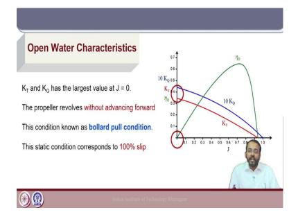
Now, let us go to the other case where J = 0; that means, the case where the propeller is only rotating without any forward velocity. In the open water case, there is no ship; so, we have considered that the propeller is rotating as well as the velocity of advance it is moving forward at V<sub>A</sub>. In the open water case, the ship is not considered and the propeller is rotating and moving at a velocity of advance V<sub>A</sub>.
