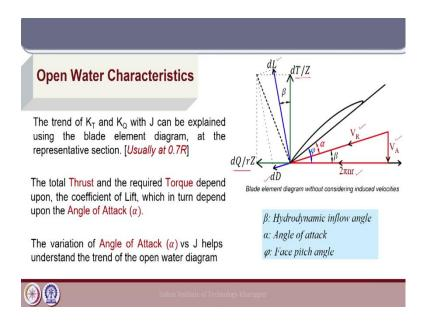
Let us explain this in the context of a representative section; so, the representative section was basically a characteristic section of the propeller blade typically at 0.7R where the characteristics of the section will be similar to that of the propeller. So, we will draw the
