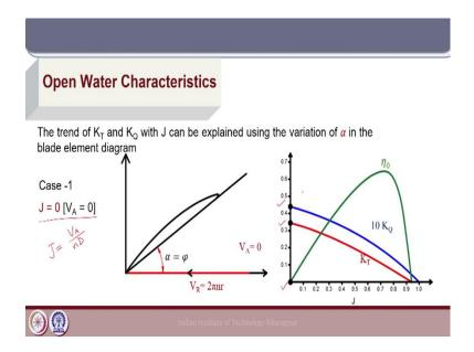
Now, let us take an extreme case of J = 0; now,  $J = V_A / n D$ . So, J equal to 0 implies that  $V_A$  will be 0; so, at that case what will be your blade element diagram like, there is no component in the axial direction. So, we have the resultant inclined at an angle  $\phi$  which is the phase pitch angle; so,  $\beta$  is 0 here, because  $V_A$  is 0. Now, this corresponds to the point on the open water diagram where J is 0.
