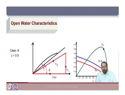
So, in this way if we go ahead to 0.7 and 0.8 the value of  $\alpha$  decreases and KT and KQ will gradually decrease. So, this gives an idea of the relation between the open water diagram to the velocities of the blade element and the resultant forces. This is very important for understanding the propeller open water characteristics. Now, we will go to the extreme cases one by one.
