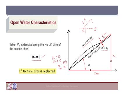
Now, on the other side what happens when  $K_T$  is equal to 0, because we have considered the case just now where the angle of attack is 0. So, even at 0 angle of attack the cambered section will provide some lift and so, there will be a small value of thrust. But how do we relate the condition where  $K_T$  or the thrust coefficient is 0 in the open water diagram, how do we relate it to the blade element diagram.
