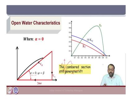
Let us take up the case where  $\alpha$  is 0, if we increase V<sub>A</sub> further such that the resultant V<sub>R</sub> is inclined to the horizontal at an angle which is equal to the phase pitch angle; that means,
