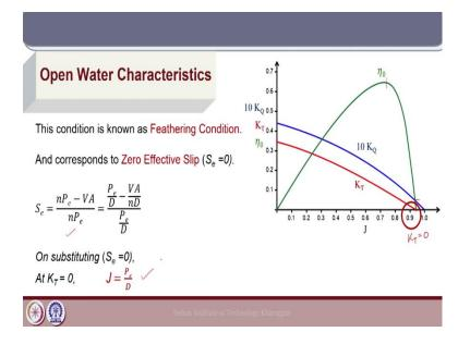
So, now let us go to this condition it is called the feathering condition where  $K_T$  equal to 0; so, again  $K_T$  equal to 0 implies that the open water efficiency will also be 0. So, in the
