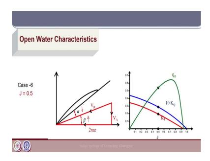
Similarly, if we go on like this from 0.3 to 0.4 we see that the angle  $\beta$  gradually increases. So, this angle  $\beta$  gradually increases which leads to the decrease of  $\alpha$ ; why? Because the phase pitch angle  $\phi$  of a particular blade section here we assume it at 0.7R which is constant. So, if we gradually increase the J the angle of attack gradually decreases and the sectional thrust and torque will decrease.
