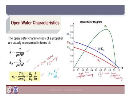
Now, let us look into the typical coefficients that we have discussed for a marine propeller. The open water characteristics are actually the plot of these coefficients for different operation conditions. So, the first one here we have the thrust coefficient  $K_T$  which is the thrust non-dimensionalized by  $\rho n^2$  diameter to the power 4 as we have seen in the dimensional analysis and the second one is the torque coefficient  $K_Q$ .
