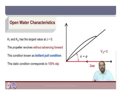
This is the blade element diagram we have already discussed where we have the highest value of angle of attack equal to the phase pitch angle.
