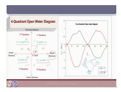
So, if we combine all these diagrams together this is what we have the 4 - quadrant of the open water diagram, we have still not shown the  $C_T$  and  $C_Q$ , but before that let us see all the components together. The 1st case  $V_A$  and n both positive, the 2nd quadrant  $V_A$  positive n negative, 3rd quadrant VA and n both negative and the 4th quadrant  $V_A$  negative and n positive.
