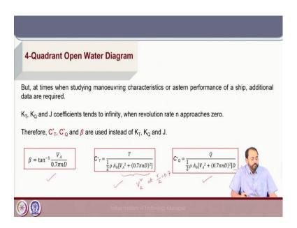
Due to some specific requirements when we do manoeuvring characteristics or calculate the astern performance of a ship, some additional data for propeller is required.
