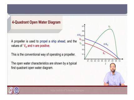
Now, we will move on to the concept of 4-quadrant open water diagram. Normally, when we plot an open water diagram it is for the case where the ship is moving ahead with the propeller rotating in a direction in which it is producing forward thrust. So, for the simple condition where we plot the open water diagram as we have seen  $V_A$  and n are both positive; that means, the propeller is advancing at a particular velocity and the propeller is rotating so, as to produce forward thrust.
