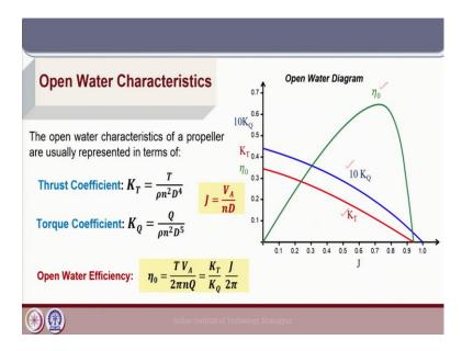
So, a brief recap of what was discussed in the last class: The open water characteristics of a propeller are the thrust coefficient and torque coefficient expressed as a function of J, where J is the advance coefficient of the propeller.
