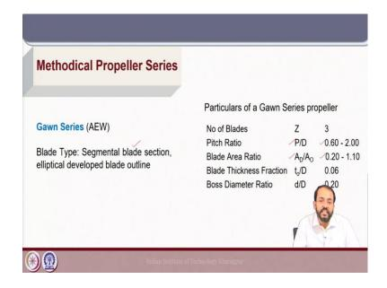
So, we will briefly look into Gawn series and B-series in terms of Methodical Propeller Series here. So, for the Gawn series the blade type is segmental blade section. So, the blade sections which are used are segmental in nature which we have discussed in propeller geometry and the developed blade outline is elliptical.
