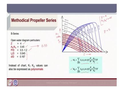
So, again just like the one that we have seen variation of pitch let us take a B-series example we have a propeller with 4 blades  $A_E/A_0$  of 0.45 and we try to see it is open water characteristics for a range of pitch ratio P/ D of varying between 0.5 and 1.2 and these factors t/ D and d/D are constants as mentioned.
