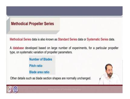
Methodical series data are used for different performance assessment of Marine Propellers. So, these are also called standard series or systematic series data which are developed based on experimentation on a number of propellers of varying characteristics.
