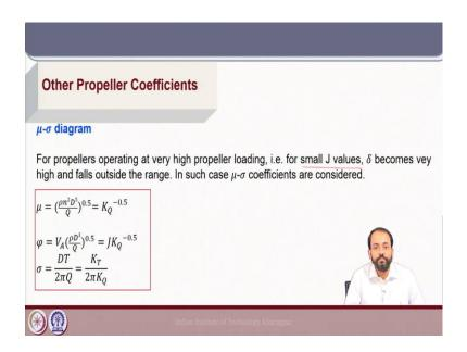
Another diagram which is used for propellers operating at very high loading is the  $\mu$ - $\sigma$  diagram. So, very high loading means we have very small J values, because the propeller loading is high when the J value is low; that means, the K<sub>T</sub> and K<sub>Q</sub> is very high. So, the thrust loading is high.
