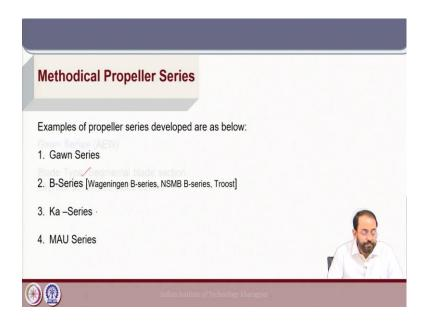
So, based on this concept certain propeller series have been developed. For example, Gawn Series the B-series or the Wageningen B-series developed at marine in Netherlands also called the Troost series sometimes, it is one of the most widely used propeller series for different purposes.
