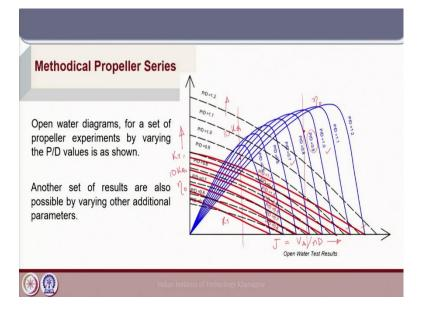
So, this is a typical example of open water test results which are obtained by varying the P/D ratio. So, if we have a particular propeller geometry and the number of blades  $a/a_0$  the blade area ratio constant, then just by varying the pitch ratio of the propeller blade we can obtain a set of curves.
