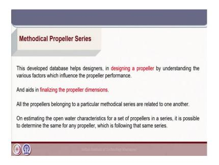
So, if we think of the database for designing a propeller certain factors are important and having a methodical series data gives a first-hand estimate to finalize the propeller dimension. So, when we discuss propeller design later in this course we will see that there are different parameters which impact the performance of a propeller.
