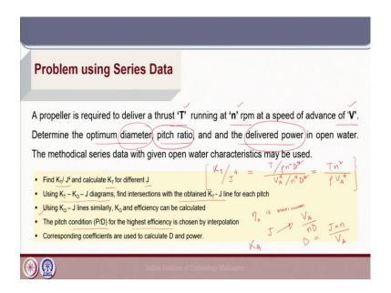
Now, if we look at a simple problem which can be done using B-series or any methodical series data. So, for this we have been asked to determine some parameters for a propeller for which the thrust rpm and velocity of advance is given. So, the requirement of thrust to be delivered at a particular rpm for a particular speed of advance is given and we have to determine the optimum diameter pitch ratio and the delivered power in the open water condition.
