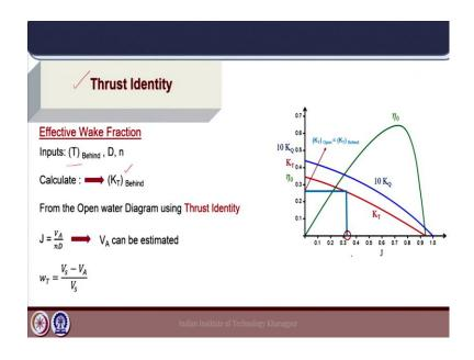
Let us look into each of these identities. First the thrust identity. Here the inputs are the thrust in the behind condition will be known. For the propeller working in behind condition the thrust is measured. And, we know the propeller diameter and rpm. Using that we can calculate  $K_T$  behind. We know the equation of the thrust coefficient. Now, using this  $K_T$  we enter the open water diagram of the propeller. This diagram is basically a plot of  $K_T$ ,
