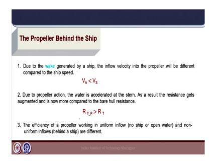
So, let us look into the basic aspects which are very important in defining certain parameters which will relate to the propulsion performance of the ship and propeller in unison. So, the first thing is the wake. When a body is moving in a fluid there is a wake generated due to the geometry of the body and the flow characteristics. And, this wake of the ship will define the inflow velocity into the propeller.
