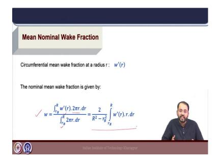
And, we can use this particular value to calculate the mean nominal wake fraction because, ultimately we want one particular value to do the estimation of ship powering. So, if we calculate the wake fraction by one particular value, it should be the averaged value of the wake fraction over the entire propeller disc, where the blades are located; that means, between the radii  $r_B$  and R.
