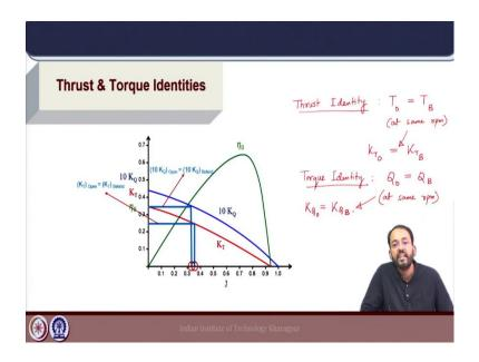
So, if we sum up the concepts of thrust identity and torque identity in a very simple way, the idea for thrust identity is that the thrust generated by the propeller in the open water and behind condition is same when it is operating at the similar rpm. That means, thrust in open water equal to thrust in behind at same rpm which gives the condition of  $K_{TO}$  equals  $K_{TB}$ .
