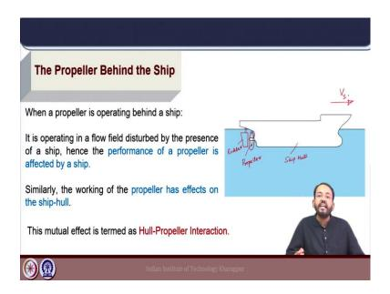
In the last week, we have covered different aspects of propeller performance in open water; that means, the propeller was working in uniform inflow condition without a ship in front of it. And, we have estimated the intrinsic characteristics of the propeller in terms of its thrust coefficient, torque coefficient and open water efficiency. Now, for a realistic condition the propeller should operate behind the ship for actual operations at sea.
