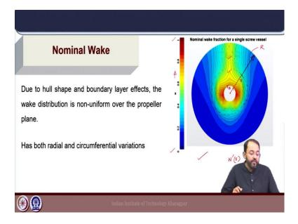
This diagram gives a plot of the axial component of the nominal wake fraction; that means, the wake fraction without the presence of the propeller and how it varies over the entire propeller disk. The value close to 1 is at the location, where the velocity deficit is maximum; that means; the blockage effect of the hull is maximum. And, the value which is close to 0; that means,  $V_A$  will be equal to  $V_S$ , where wake fraction is 0; where the flow is equal to the free stream velocity.
