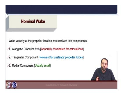
So, the different components of nominal wake are the three components. One in the axial direction which is the most important component and that is used for the propeller calculations. Because, the axial component of the wake fraction is what impacts the  $V_A$
