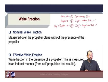
Now, these three effects create a difference between the forward speed of the ship  $V_S$  and the speed of advance of the propeller  $V_A$ . The difference is called the wake fraction which is expressed as a non-dimensional fraction divided by the forward speed of the ship. So, there are two ways of defining wake fraction.
