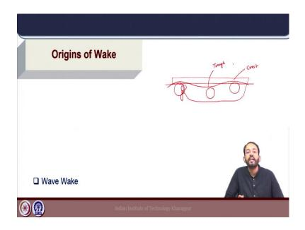
The third factor here is the wave wake. So, if we look into the location of the propeller behind the ship. The ship due to its motion forward at a particular speed creates a wave and this particular wave generated by a ship, this wave pattern depends on the Froude number of the ship. Due to this wave making pattern of the ship which is Froude number dependent or; that means, it is forward speed dependent, the wave pattern will impact the particle velocities just below the wave.
