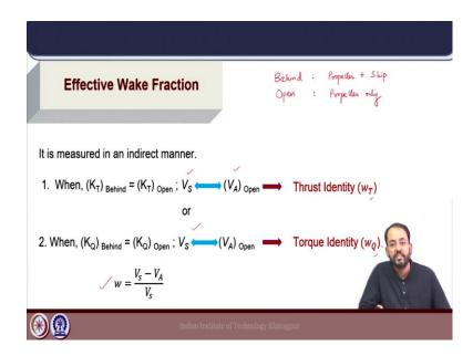
Now, we will move on to the effective wake fraction; that means, the wake fraction when the propeller is working behind the ship. In this particular case, we do not measure it directly. It is estimated in an indirect way; that means, we use the different identities, the thrust and torque identities using the results of the self-propulsion test and the open water test.
