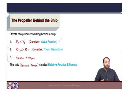
Now, if we look into these effects, the first one is the velocity of advance is lower than the ship speed and this leads to the consideration of wake fraction. The increase of resistance due to propeller action with respect to the total resistance measured during the resistance test is taken care of by a factor called thrust deduction. And, the difference in efficiency between the behind and open condition is taken care of by a factor called relative rotative efficiency.
