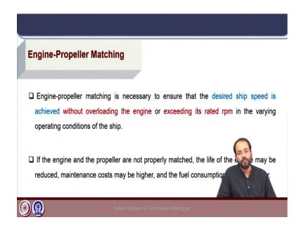
Now, the engine propeller matching needs to ensure that the desired speed is achieved without overloading the engine or exceeding its maximum rpm for varying operation conditions of the ship. If they are not matched properly what can happen? The engine life span may be reduced because of sub optimal operation conditions and also maintenance costs may be high, the fuel consumption may be high which will affect the economy of the vessel.
