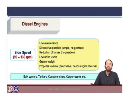
So, if we look into the aspects of slow speed diesel engine these are low maintenance and very simple arrangement because the engine is directly connected to the propeller. So, direct drive is very much possible here and there is no gearbox involved. So, the engine being directly connected to the propeller, the rpm of the engine will be same as the propeller here.
