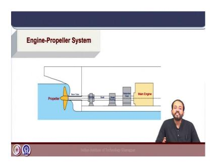
This diagram shows the engine propeller system for a ship which was shown in hull propeller interaction class and here we have the main diesel engine which is connected to the propeller via a shaft. And there is a reduction gear shown which I mentioned is optional depending on the type of engine and the thrust bearing is transmitting the thrust which is generated by the propeller to the hull. So, now we will move on to the different types of engines or propulsion plants, which are used in ships.
