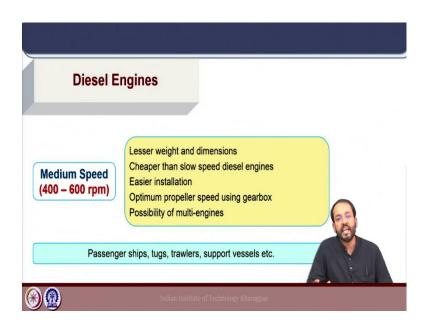
Next the medium speed diesel engines which operate in the range of 400 to 600 rpm in general. So, the weight in this case is lower and the dimension also smaller compared to slow speed engines. They are cheaper than slow speed diesel engines and installation is easier because of smaller dimensions.
