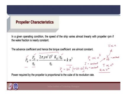
Now, let us consider the propeller characteristics. What is the nature of the propeller with respect to the relation between the power and the rpm? In general, it can be expressed as a cubic function that the power is proportional to  $n^3$ , we can write  $P_B = k n^3$ . Now, what is the logic behind this and what are the implications? So, for a particular operation condition it is observed that the ship speed is almost linearly varying with the propeller rpm.
