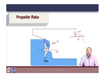
What we get is the path will be a helicoidal, but with an angle. So, this will be the generated path the screw propeller generated from such a line will have a rake. Now why is rake given to a propeller? The first one the propeller had in the earlier picture had no rake in this particular case. So, rake is 0 rake angle is 0.
