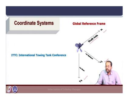
Now, the International Towing Tank Conference which is basically an association of organizations which deal with ship hydrodynamic testing. They have defined a global reference frame for ship propeller system and these ITTC norms are heavily used for experimental testing of model ships and propellers and also for numerical analysis of ship hydrodynamic problems.
