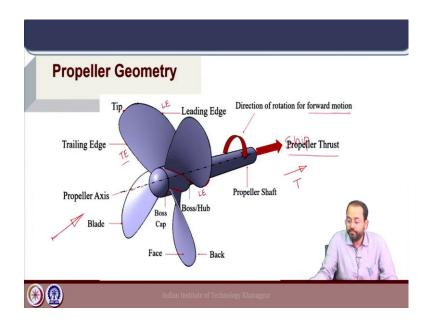
So, this is the geometry of a standard screw propeller where a set of blades are mounted on a central structure called the boss or hub which is connected by shaft to the marine engine. So, let us look at it one by one, we have the propeller shaft which is connected to the marine engine, and where through which the power is delivered to the propeller.
