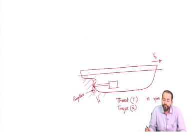
The basic thing which is very important to understand is the location of the propeller with respect to the ship. So, this is the ship let us say which is moving forward with the velocity  $V_s$  we have the propeller which is located in the stern of the ship. So, here we have the propeller. Now, the propeller is connected by a shaft to the marine engine which provides the power which is delivered to the propeller for its rotation.
