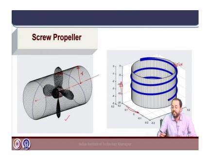
Now for the same diagram if we see multiple turns now you can visualize the helical surface in a better way ok, as it moves along the cylinder.
