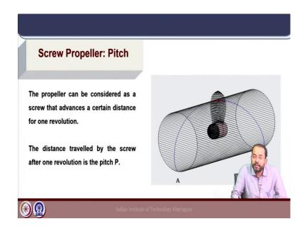
Now a screw propeller can be considered as a screw that advances a certain distance for 1 revolution ok. Now, the distance travelled by the screw after 1 revolution is called the
