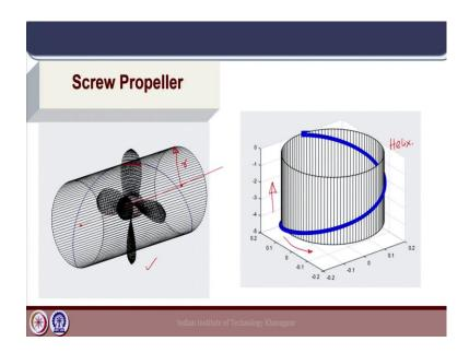
Now, why is a propeller called a screw propeller? As we have seen in the introduction class that the basis of a screw propeller comes from the concepts of Archimedean screw; that is screw having a certain pitch as it rotates along. Now when we have a screw it rotates along a central axis and it also moves forward.
