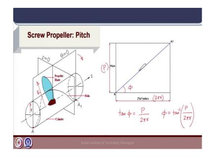
Now, if we try to visualize putting a set of axis on this entire diagram, we have the cylinder and we try to develop a very simple coordinate system which is basically the cylindrical coordinate system defined by r,  $\theta$ , and z. Now, z is along the axis of the propeller here r is simply along the radius of the cylinder, and  $\theta$  is defined with respect to the vertical.
