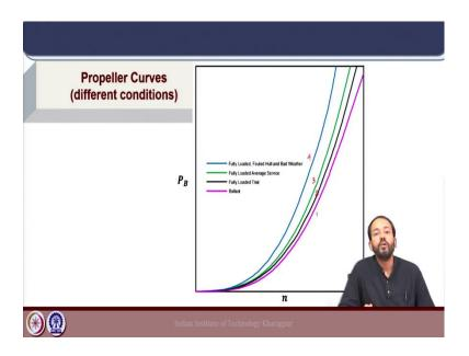
So, we have discussed different propeller curves for different operation conditions for a ship. We have the ballast condition for which the power demand is lowest, the first curve from the bottom here. Next, we have the fully loaded trial condition, the black line where the powering demand will be higher as compared to the ballast condition.
