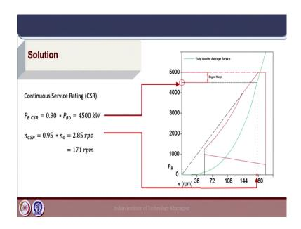
Now, the continuous service rating is 90 percent of the maximum power and here, we can see that the fully loaded average service condition can be intersected with the engine diagram and we can see that the point for continuous service rating can be obtained here. And the rpm at continuous service rating as per the given problem is 95 percent of the maximum rated rpm, which is 171 as shown here ok.
