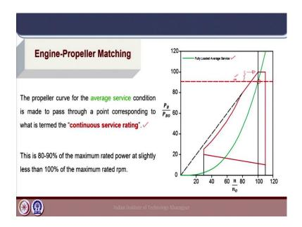
Now, what is the basis of engine propeller matching; how do we place the propeller curve in perspective to the engine curve? This is the question which I had asked in the last class and the basis for that will be the continuous service rating. What is typically done here is the average service condition of the propeller curve is taken.
