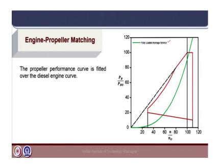
So, for the propeller power curve, the condition of fully loaded average service is taken and that propeller curve is juxtaposed on the engine performance curve. The reason for choosing this will be discussed later, when we talk about the margins and in this way we have to understand the relation between the propeller power demand and the power generated by the engine when we do the engine propeller matching.
