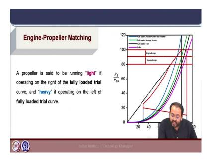
Now, if the propeller is operating on the right of the fully loaded trail curve; that means, we have this black line which is the fully loaded trial curve, if the propeller operates to the right of that curve; that means the powering demand is lower than the trial condition that is considered as a light running condition.
