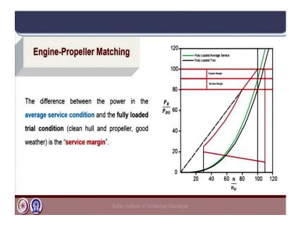
Now, there is one more margin which is required. Basically, it is the difference between the power demand in the average service condition and the fully loaded trial condition. So, in these set of curves, we add the next condition for the propeller which is the fully loaded trial condition in addition to the average service condition, which is already shown.
