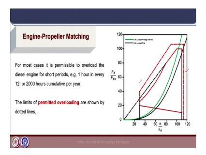
Now, for most cases, it is permissible to overload the diesel engine for very short period; that means the diesel engine can be operated beyond the maximum rated values. So, overloading is applied, but for only very short period; that means, 1 hour in every 12 hours as a standard or 2000 hours in a cumulative way per year.
