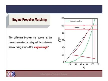
This margin is called the engine margin. So, the maximum rated condition is the MCR of the engine and the continuous service rating CSR is the point, where this fully loaded average service condition intersects with the engine curve which is slightly lower than the maximum continuous rating. So, the difference between them is called the engine margin ok.
