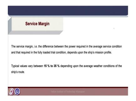
Now, the service margin which is the difference between the power demand between the fully loaded trial condition and the average service condition will depend on the operational characteristics of the specific ship type. Now, this can have a value of anything between 15 to 35 percent depending on the average weather condition on the ships route.
