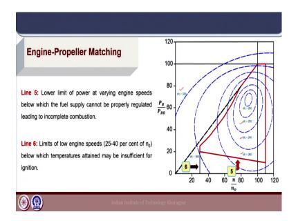
Line 5 is the lower limit of power at varying engine speeds. So, this line gives the lower limit below which the fuel supply cannot be properly regulated, which will lead to incomplete combustion of the fuel and the performance of the engine will not be proper. And finally, line 6 is the limit of low engine speed below which the temperature attained will not be sufficient for ignition.
