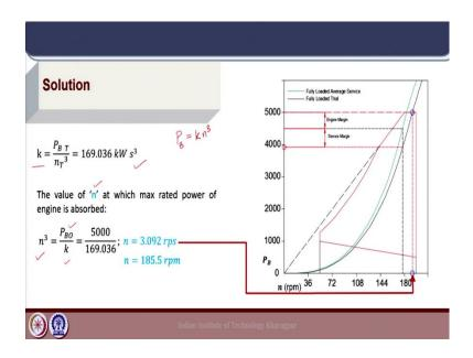
Now, for the propeller, we know that the assumption for the propeller power demand proportional to the cube of propeller rpm is used for engine propeller matching. So, we have to find that factor k, where  $P_B = k n^3$  ok. We have calculated the  $P_B$  in the trial condition,  $P_{BT}$  and the rpm in the trial condition is also known. So, from that, we can calculate k. It will have units based on  $P_{BT}$  and n.
