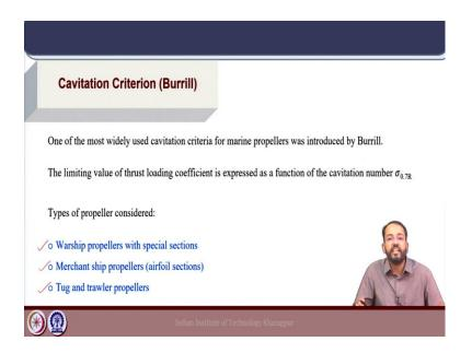
Now, we will look into a cavitation criterion that is used for marine propellers and extensively used for propeller design to get a design within a certain range so that the probability of cavitation occurrence is minimized. One of the most widely used criteria was proposed by Burrill and it is expressed by the thrust loading coefficient of the propeller blade as a function of the cavitation number at 0.7R which is the reference section.
