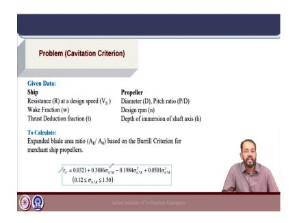
Now, we will do a simple problem of cavitation calculation on a propeller blade using Burrill's cavitation criteria. In this problem we have the ship data given where the resistance of the ship at a particular design speed is given along with wake fraction and thrust deduction fraction.
