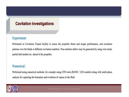
Now, what are the standard ways of cavitation investigation on propeller blades? We have briefly covered the concept of cavitation tunnel under model tests. So, cavitation tests are done in cavitation tunnel facility where the propeller thrust and torque performance as well as cavitation patterns are studied at different cavitation numbers.
