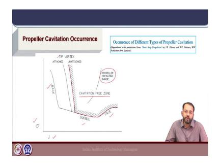
Now, here we will see the different types of cavitation occurrence with respect to a propeller operation. So, initially we have seen very simply the concept of cavitation bucket for a 2D foil section and how the effect of thickness govern the formation of different types of cavitation. Here the same is studied in the context of a standard propeller blade.
