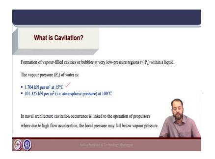
So, just a brief recap of the cavitation phenomena – it is the formation of vapor filled cavities or bubbles at very low pressure within the liquid. And, we have seen for naval architecture application like ship propellers. It is possible that the local velocities may be very high due to flow acceleration around the propeller and that can lead to the local pressure falling below the vapour pressure and, the vapor pressure for water at 15 degree is 1.7 kilonewton per meter square.
