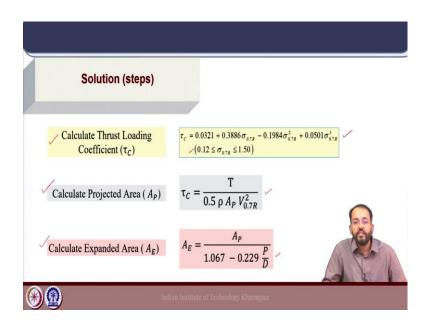
Next, we can calculate the thrust loading coefficient; for merchant ship propellers. The equation is already given for cavitation criteria because we have already computed the cavitation number the thrust loading coefficient can be obtained using this expression and we will see that the calculated cavitation number if it is given for a merchant ship propeller it should lie within this particular range.
