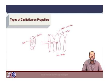
For propeller blades, we have seen different patterns of cavitation depending on both the type as well as its location on the propeller blade. So, if we have a propeller blade here, it can happen that due to high angles of attack combined with higher velocities on the propeller blade a certain portion on the blade can have a sheet of cavitation happening over the suction side typically.
