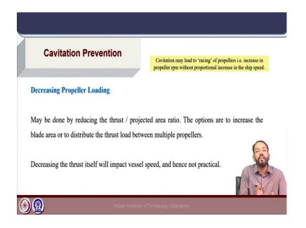
So, what other options do we have? We can decrease the propeller loading. So, if the thrust loading of the propeller is decreased; that means, the thrust per projected area ratio which is standard used for propeller blade cavitation calculations. So, if that is reduced we have seen that the cavitation occurrence is higher at high thrust loading conditions.
