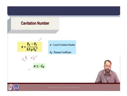
And, we have already defined the cavitation number using this expression where  $P_0$  is the reference pressure and  $P_V$  is the vapor pressure at the particular temperature. Now, here if we see the reference velocity is  $V_0$ , and we have seen that this reference velocity depends on the way the cavitation number is defined for the propeller. So, typically for a representative section of the propeller blade this will be the resultant velocity at 0.7 R for the propeller blade.
