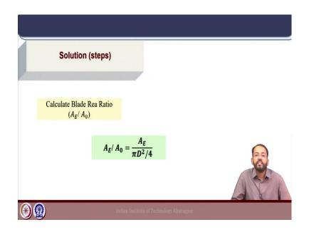
Next the final step from the value of expanded blade area as discussed in propeller geometry we can divide it by the area of the propeller blade, the disc area  $\pi D^2/4$  where D is the propeller diameter to get the expanded blade area ratio  $A_E/A_0$ . So, the same problem can be framed in different way the idea is to calculate the parameter of a propeller based on cavitation criteria.
