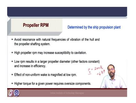
Now, let us look into the next consideration, which is the propeller rpm. This propeller rpm is typically determined by the ship propulsion plant and the matching of the propeller with the particular engine chosen for the ship is very important in terms of propulsion efficiency. And the engine should also perform at its optimum level along with the propeller for a optimum performance of the ship propulsion system together.
