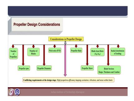
Let us look into some general considerations, which are of prime importance in propeller design. The first consideration here is the number of propellers. Now, for a specific type of vessel based on design experience, often the number of propellers is chosen by default. That means, based on experience of designing similar types of ships based on their operation conditions and thrust loading the number of propellers is chosen.
