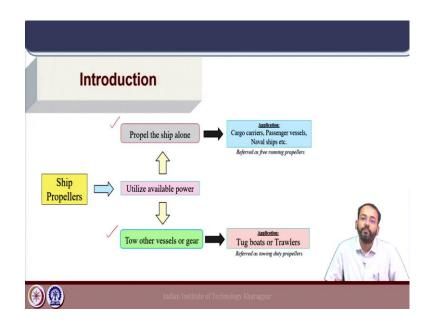
So, if we look into ship propellers; their main function is to utilize the available power, which is delivered from the engine and develop the thrust required to propel the vessel forward. That is the main purpose of ship propellers. And as discussed here we are considering skew propellers. There are other types of propulsion systems for ships which we will discuss in the later lectures.
