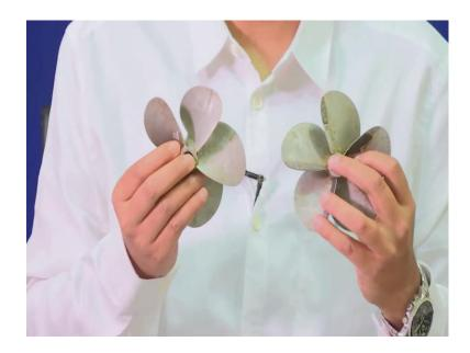
This is a model propeller which we use for testing in the towing tank, where we test the propeller; open water characteristics as well as the behind hull performance to estimate ship powering. So, this model is made to a particular scale as per the requirement of the testing. Here we see that you have a central part which is the hub; on this hub the blades are mounted. In this particular case of the propeller, it is a 5 bladed propeller.
