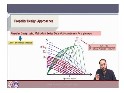
Now, again the similar process will be involved. The only change with respect to the previous process is instead of the line which represented  $K_T/(J^2 \times J^2)$  in the initial process where rpm was not known here, because we have the diameter as unknown we use  $KT/J^4$  which is given by this expression and multiply with  $J^4$  to get the  $K_T$ .
