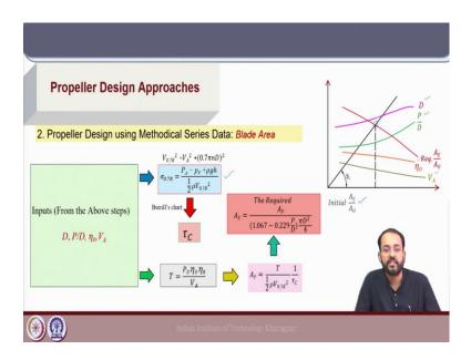
So, the inputs for this calculation will be the propeller diameter, pitch ratio open water efficiency and  $V_A$  are known. Next, we calculate the cavitation number for the representative section at 0.7 R on the propeller blade. The details have been discussed in the lecture under propeller cavitation.
