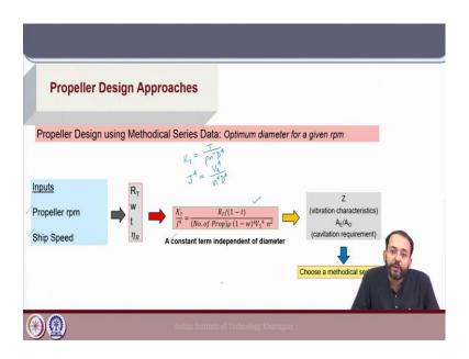
In the second approach we will look into the design problem in just the opposite way; that means, for a given propeller rpm we will use the same design charts to obtain the optimum propeller diameter.
