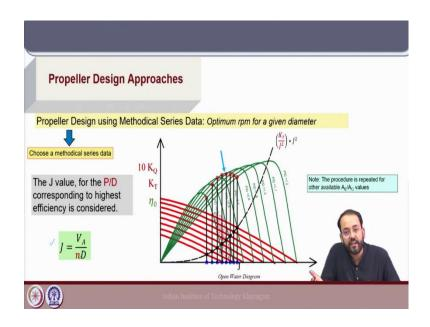
Finally, we will choose the J value for the P/D for which we are getting the highest efficiency and we can see here that the highest efficiency is corresponding to this particular point.
