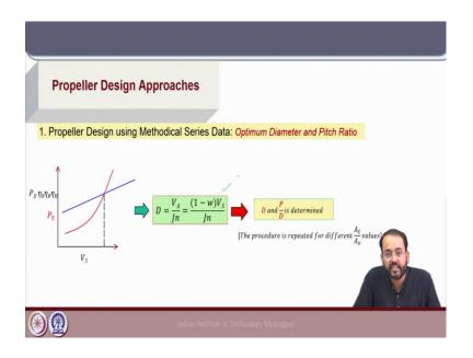
Next, we get the particular design point and for that specific case we calculate the propeller diameter based on this expression. Because in this particular problem the propeller diameter is an output of the design process and in this manner the diameter and pitch ratio of the propeller is determined in the design process.
