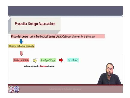
And from that we can get the power of the propeller because corresponding to the maximum efficiency again we can calculate the  $K_Q$  and we can calculate the torque and finally, the delivered power of the propeller. So, these methods give an initial estimate for the basic parameters like diameter and rpm of the propeller design and the delivered power required for the particular design.
