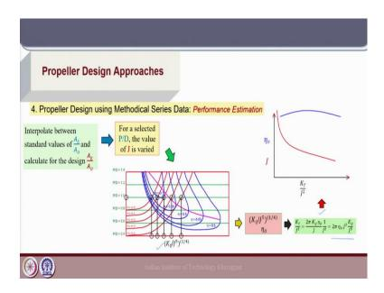
Finally, we will do the performance estimation for the propeller. Now, here we have the standard  $A_E/A_0$  values for the specific series and we calculate these parameters for the design  $A_E/A_0$  values, which is already done. And here for the selected P/D value we will vary the value of J in the propeller curves which are shown here for the different J values, here denoted as one by J for the given P/D which is the design P/D which is obtained now. We get different  $K_0/J^5$ .
