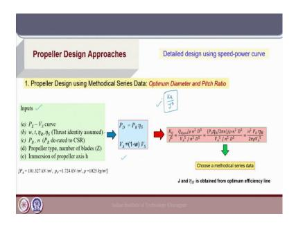
Now, for the detailed propeller design procedure using methodical series data, a series of input parameters are used. The first one being the effective power versus speed curve for the ship for which we are designing the propeller.
