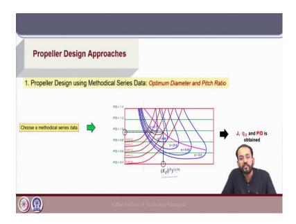
In this method we will use a different version of the open water charts where this expression is related to 1/J for different P/D ratios for the propeller and this pink line shows the optimum efficiency line.
