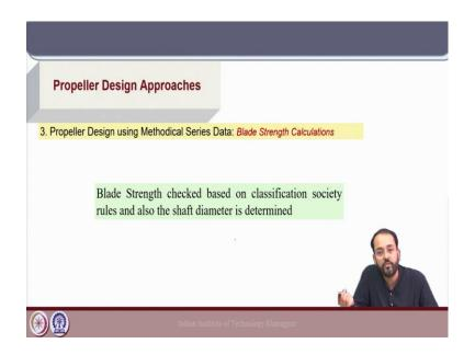
So, next the blade strength needs to be checked. Here the interesting part of the design process is whatever we have learnt under different parts, the calculation of thrust torque efficiency from the open water diagram, cavitation blade strength everything will be used in the design process to get the final design of the propeller which corresponds to an optimum value of efficiency and satisfying cavitation and strength requirement.
