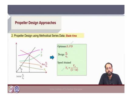
So, we use the same set of curves here to get the optimum diameter P/D ratio and design  $A_E/A_0$ . And finally, the attained speed for that specific blade area ratio is given by this expression.
