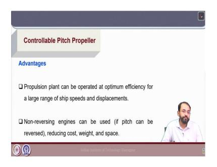
Next, if we have a controllable pitch propeller, the propulsion plant can be operated at optimum efficiency for a large range of ship speeds and displacements. So, it can happen that the displacement can change over different operation conditions and due to change in the ship speeds also, the efficiency of the propulsion plant will change depending on the engine propeller matching, if we have a fixed pitch propeller.
