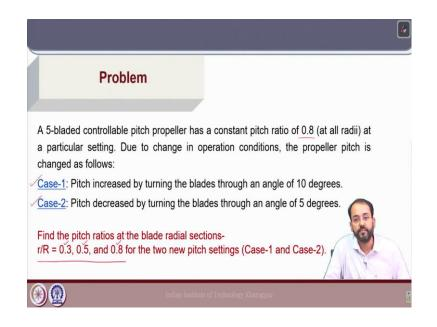
Now, let us look into a simple problem which explains the change in pitch distribution due to the change in the pitch for a controllable pitch propeller. So, in this problem, we have a 5-bladed controllable pitch propeller which has a constant pitch ratio of 0.8 at all radial locations on the propeller blade for a particular pitch setting. So, this specific propeller has a constant pitch ratio for all radial locations on the propeller blade given at a particular setting.
