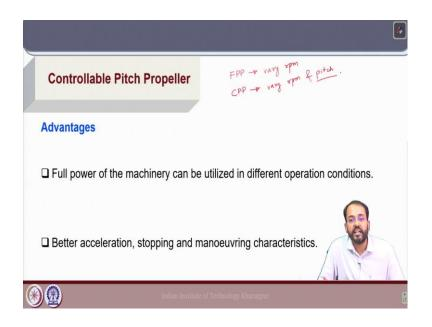
Now, we will discuss some basic advantages of controllable pitch propellers. The first advantage mentioned here is that the full power of the propulsion machinery can be utilized in different operation conditions. So, if we have a fixed pitch propeller, we can only vary rpm. This we have just seen and for controllable pitch propellers CPP, we can vary both rpm and pitch. Now, for some ships, there are shaft driven generators, where there is a requirement to maintain a specific rpm.
