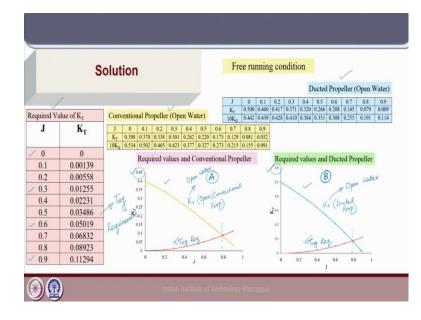
So, this particular table shown here is the same table which was calculated in the last slide and this forms the required thrust coefficient for different operation conditions. And here we have the two open water diagrams, one for the conventional propeller and another for the ducted propeller. And from each open water diagram we can have a thrust coefficient versus J curve and we can match that with the required value of thrust for the tug. So, this table gives the tug requirement.
