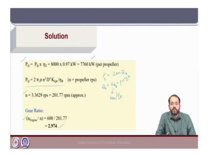
So, the first step will be to calculate the delivered power because we have to compute the propeller rpm. So, the delivered power can be easily calculated from the brake power of
