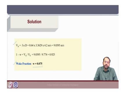
Next, we have to calculate the propulsion factors. Now, for the given value of J we can calculate the advance speed  $V_A$ , and because the shift speed is known we can simply calculate the wake fraction by comparing the advanced speed with the ship speed. Here, we should note that the wake fraction is very low because this is a twin-screw ship. And it is expected here that the value of wake fraction will be less than 0.1.
