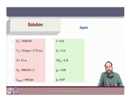
So, let us look into the inputs, the effective power, the design speed, the diameter of each propeller for the twin-screw ship, the brake power of each engine and the engine rpm. And on the propeller side for the given advance coefficient, the thrust and torque coefficients are provided and the relative rotative efficiency and shafting efficiency are given.
