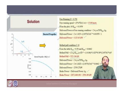
Next, we do the same calculations for the ducted propeller. Here also we find the point of intersection between the  $K_T$  curves from the tug requirement, the red line, and the  $K_T$  curve for the propeller. And we see that for this particular problem the data is given in such a way that they intersect at the similar value of J which is 0.79 and that gives a free running speed of 15.8 knots which is same as for the other case.
