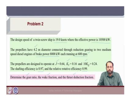
Let us look into another problem where we have a twin-screw ship of design speed 19 knots where the effective power requirement is provided. And it has propellers of 4.2 meter diameter and because it has medium speed diesel engines, reduction gears will be required as the propeller rpm will be different from the engine rpm. And the brake power of these engines two of them is provided and the engine rpm is also provided.
