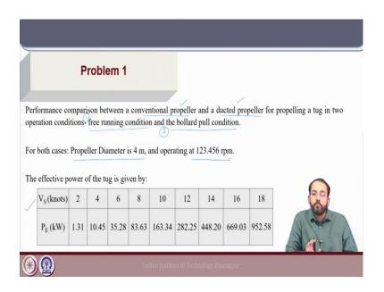
For the first problem, we are given a tug for which we have to do a performance comparison between a conventional propeller and a ducted propeller for two different operation conditions. 1 is the free running condition and number 2 is the bollard pull condition. So, we have a tug with given effective power versus speed curve and using this data, we have to apply the details of the propeller diagrams.
