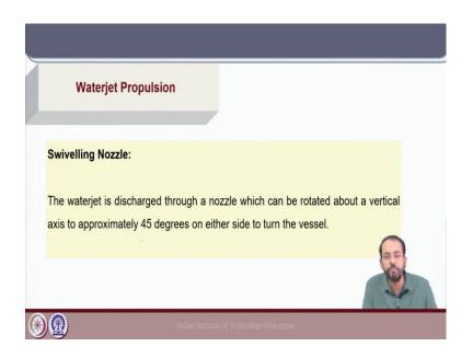
The swiveling nozzle which is present at the exit of a waterjet system can be rotated about a vertical axis to approximately 45 degrees on either sides to turn the vessel and that is how the jet is deflected on the port and starboard sides and the vessel can be maneuvered accordingly.
