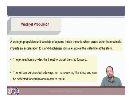
The waterjet propulsion system is one of the earliest forms of mechanical propulsion systems installed in ships. It has been used as early as in the 17th century to propel ships using different types of pumps installed at the stern of ships and they used to provide the thrust to propel the ship forward. Now the modern version of a waterjet propulsion unit consists of a pump which is housed within the ship.
