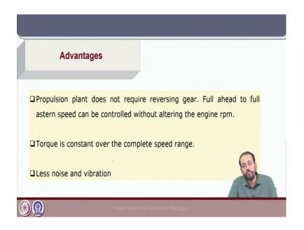
In waterjet systems there is no reversal gear required due to that the full ahead to full astern speed can be controlled without operating the engine rpm. Torque is constant over the entire speed range because we are not changing the engine rpm and this leads to optimal performance in terms of the specific fuel consumption and less noise and vibration because the impeller is working within the hull enclosed in the waterjet system. So, the noise and vibration levels are lower.
