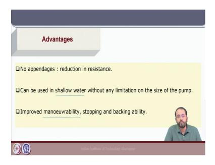
Now, if we look at the advantages the first advantage mentioned here is we do not require any appendage because the entire waterjet system is housed within the stern of the ship. So, there are no appendages like brackets or other structures which are otherwise required for conventional propellers.
