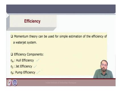
Regarding the efficiency under normal thrust loading conditions a waterjet propulsion system will have in general a lower efficiency as compared to a conventional propeller. So, these are used for vessels where the speed is generally quite high typically above 30 knots and it is fitted specially in ferries and naval vessels, where the requirement of thrust is high and maneuverability is very good.
