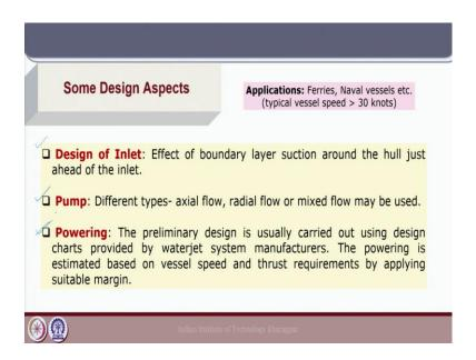
In terms of application, waterjet propulsion systems are used in ferries and naval vessels typically fast attack crafts, where the vessel speed is higher than 30 knots and waterjets give very good performance in terms of maneuverability and other operation conditions for these ships. Now, we will briefly look into some design aspects which are critical for waterjets.
