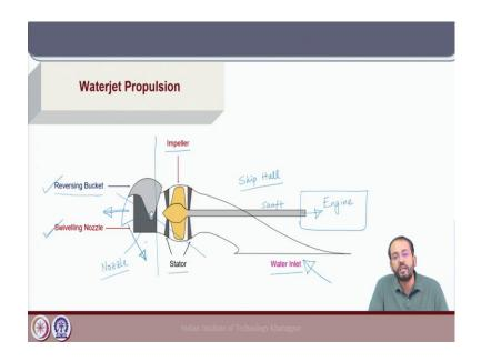
Now, let us look into the components of a waterjet propulsion system. We have the water inlet here through which the water is being drawn into the waterjet propulsion system and we have the nozzle here which is swiveling in nature. That means it can be rotated in either ways. This nozzle is throwing the water from the stern of the ship.
