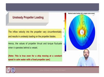
Let us start with the first topic which is unsteady propeller loading. The inflow velocity into the propeller varies circumferentially at each radial position on the propeller blade, and we have seen how the wake varies at the propeller position due to the presence of the ship hull.
