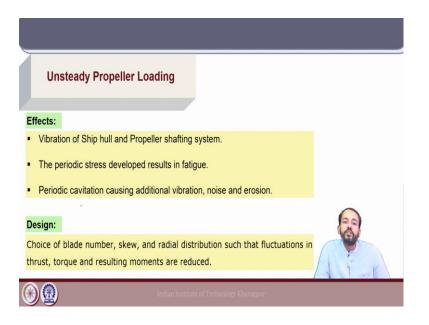
Now, what are the effects of unsteady propeller loading we have vibration of the ship hull and propeller shafting system. The periodic stress which is developed on the propeller blade that results in fatigue during the life cycle of a propeller as it is operating in the sea conditions, and periodic cavitation, which causes additional vibration noise and erosion.
