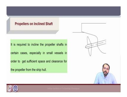
Next, we will look into propellers on inclined shaft. For certain ship designs it is required to incline the propeller shaft, especially in small vessels where sufficient diameter is not available. So, in order to maintain the clearance from the ship hull the shaft of the propeller is inclined, and because of that a greater space can be obtained for the propeller in the stern of the ship.
