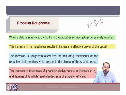
Next, we will discuss propeller roughness. When a ship is in service, both the hull as well as the propeller surface will get progressively rougher due to its operation in the marine environment, and corrosion will also occur. And, this increase in roughness will result in the increase of effective power of the vessel.
