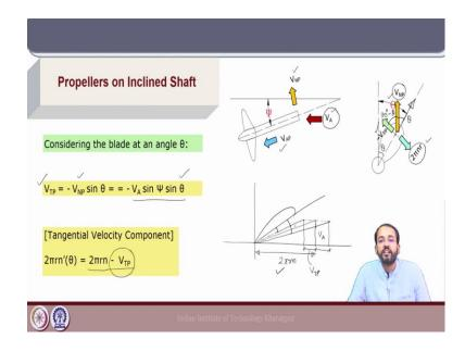
Now, let us consider the case of a propeller which is on an inclined shaft and the instantaneous position of one of the propeller blades is at an angle  $\theta$  with respect to the vertical 12 o' clock position. So, we have this V<sub>AP</sub> which is the axial component due to the velocity V<sub>A</sub> and V<sub>NP</sub> which is the normal component for the case of an inclined shaft propeller.
