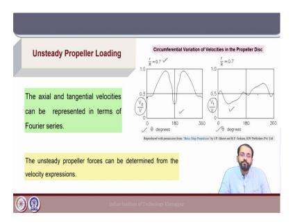
Now, the variation of axial and tangential velocities over the entire circumference location of the propeller disc based on the variation in theta is shown here. For the axial component it is non-dimensionalized by the inflow velocity V and similarly the same is done for the tangential component.
