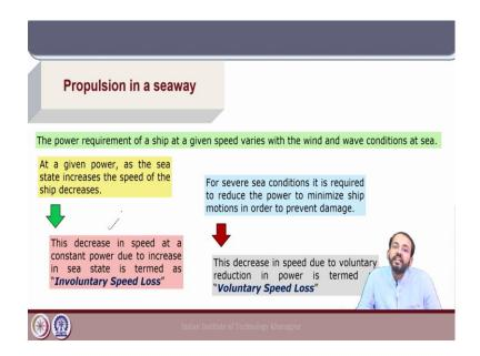
Next, we will discuss propulsion in a seaway. The powering performance of a ship for a specific speed will vary with the wind and wave conditions at sea. And, hence the sea condition which is typically given by sea state will decide the powering performance of a vessel in an actual operation condition.
