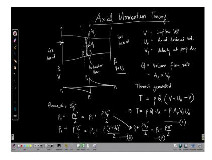
Let us take a flow domain where we have the propeller disc or the actuator disc as we say. So, here we have the actuator disc which is basically giving the thrust here. So, we have taken the domain so that it extends far ahead of the disc and to a zone which is far behind. Now, what are the pressure and velocity components in these regions? Far ahead let us say it is pressure is  $P_0$  and a velocity we put at the inlet which is in this direction which is V.
