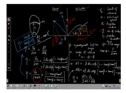
Now, using equations 3 and 4, ok efficiency can be written as  $V_A/2 \pi n \times (Z dL \cos(\beta) (1-\tan(\beta)\tan(\gamma)) / (r Z dL \cos(\beta) \times (\tan \beta + \tan \gamma)))$ , ok. So, this efficiency becomes Z dL  $\cos(\beta)$  is cancels out, so it is  $V_A/2 \pi r n \times (1 - \tan(\beta)\tan(\gamma)) / (\tan \beta + \tan \gamma))$ , ok. Now, one final line; what is this fraction  $V_A/2 \pi r n$ ?
