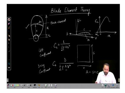
Now, let us try to look into the different aspects of the blade element theory. So, we have the propeller blade. This is the radius of the propeller blade R, and the blade is fitted over the boss or the hub. This is the radius of the  $hub(r_h)$ ,. And let us take any cylindrical section at a radius small r, of thickness dr, ok. So, this is basically the blade element.
