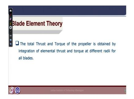
And then, the total thrust and torque of the propeller blade can be obtained by integration of this elemental thrust and torque at this radii. So, what we do is, we for each element we can compute the thrust and torque of the propeller and then we can integrate them over the blade, over the part of the blade which is producing. So, that from the hub to the tip and then that gives us the total thrust and torque of the propeller, ok.
