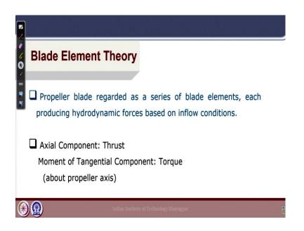
So, before going into the details let us try to understand what are the assumptions of the propeller blade element theory. In this theory, we have the propeller blade which is regarded as a series of blade elements. Initially, we have started with the most simple theory which is the axial momentum theory where the propeller blade was not considered.
