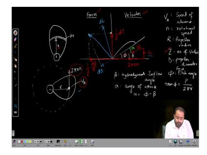
For this case, what will be the forces based on the velocity at that particular section? Now, if I look at a propeller blade, it is rotating as well as moving ahead. Here we have a case where we have a velocity which is coming to the propeller blade which is the inflow velocity or as the propeller blade is advancing, so it is a velocity of advance, we call it  $V_A$ .
