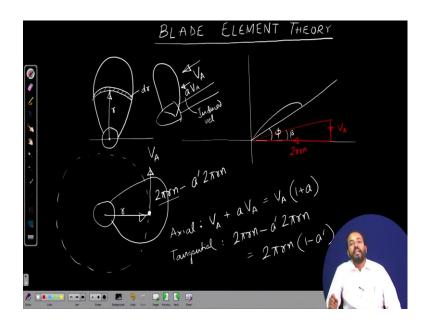
Now, let us move. Now let us start with the blade element theory considering induced velocities. Similar to the basic blade element theory calculation we have a propeller blade for which we are taking a small strip or the element at a radius r of thickness dr ok and for that element we will try to compute the thrust and torque. So, again we will draw the blade element diagram. So, using the same nomenclature we have used for the basic blade element computations.
