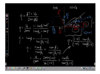
Efficiency is given by thrust into velocity of advance by 2  $\pi$  n × torque (Q) ok. So, everything with a d here because we are computing the efficiency of the propeller blade section ok. So,  $\eta$  will be V<sub>A</sub>/2  $\pi$  n ×d T/d Q. So, Z dL cos $\beta_1$  cancels out we have only the tan part and r (1- tan( $\beta_1$ ) tan ( $\gamma$ ) / (tan ( $\beta_1$ ) + tan ( $\gamma$ )) with an r ok.
