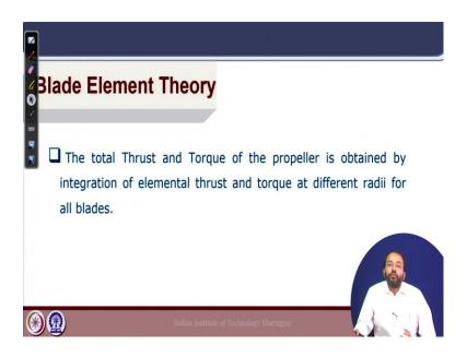
And the total thrust and torque of the propeller blade can be obtained by integrating the elemental thrust and torque at different radius for all the blades.
