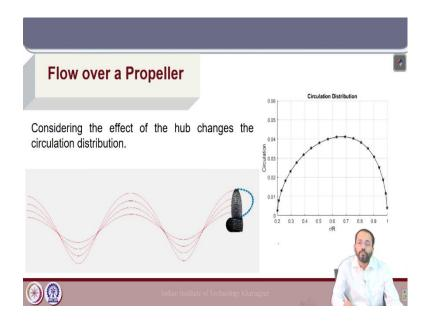
Now, if we consider the effect of the hub, then the circulation distribution will be slightly different. So, this is the original circulation distribution from the root of the blade to the tip.
