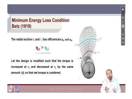
Now, one important aspect for a propeller is the minimum energy loss condition proposed by Betz. Let us take 2 radial locations of the propeller blade at two sections at radius  $r_1$ and  $r_2$ , where the ideal efficiency are  $\eta_{i1}$  and  $\eta_{i2}$ . And we assume that we have taken the sections in such a way that the ideal efficiency at  $\eta_i$ ,  $\eta_1$  at the location  $r_1$  is greater than at location 2. So,  $\eta_{i1}$  is greater than  $\eta_{i2}$ .
