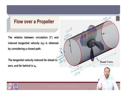
Now, let us try to understand the relation between the circulation and the induced velocity for a propeller blade, because the induced velocities impact the resultant velocity distribution on the propeller blade and finally, the thrust, torque and efficiency of the propeller ok.
