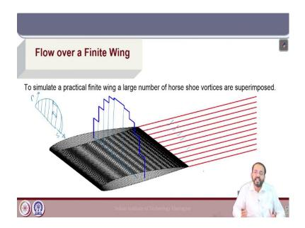
So, if we divide the finite wing into a number of elements, the circulation distribution is 0 at the ends and maximum at the center. So, if we divide this into a number of elements, this span then the circulation gradually increases towards the center of the span.
