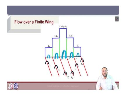
So, in the next figure we will see how it increases accordingly from one element to another. We have  $\Gamma_1$ , the circulation at the two ends due to the actual trailing vertices from the two ends. So, gradually as we go a very few number of elements is shown just to diagram show how the circulation increases towards the center of span.
