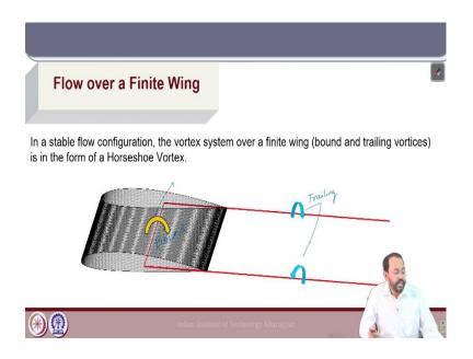
In the last class we have covered the key aspects of circulation related to a finite wing. So, from the concept of an airfoil we would now try to develop the concept for circulation around a propeller.
