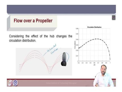
If we consider the effect of the hub the circulation will not be 0, at r/R of 0.2 here we take that the hub radius we take it as 20 percent of the propeller radius. So, it will have a finite value, because now considering the hub that part of the blade does not end in fluid.
