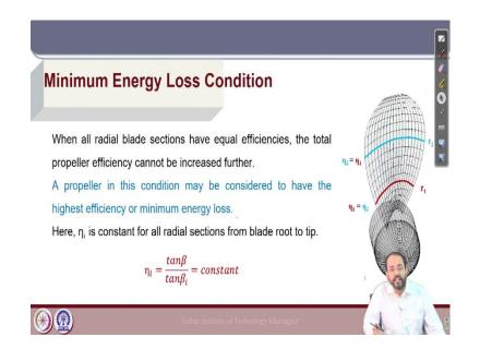
Now, what do we understand from this? So, whenever two blade sections have different efficiency, we can modify the sectional characteristics, the pitch distribution to change the efficiency in such a way that the thrust will increase, but the torque will remain same in a way so that the final efficiency will increase. So, we can continue doing this exercise till all the sections will have the same efficiency.
