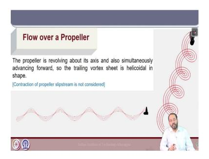
This is a representation of the vortex sheet, trailing edge vortex sheet behind the propeller and it should be noted that we have not considered the contraction of propeller slip stream in this case.
