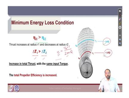
What we will see? Here the torque change at  $r_1$  is by  $+\Delta Q$  and  $r_2$  by  $-\Delta Q$ .
