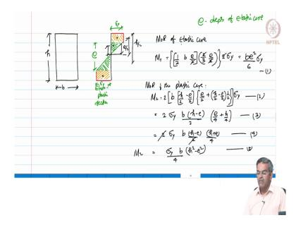
The cross section has the dimensions b and depth as d. Let us h, let us design a hybrid section where the section is partially plastic and the remaining is elastic. Let us have an elastoplastic section. So, let us have an elastoplastic section.
