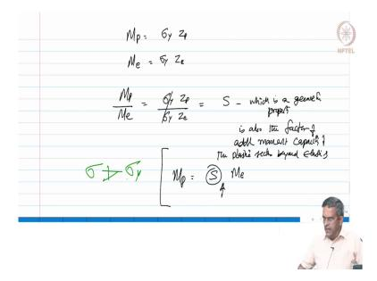
Let us say  $M_p = \sigma_y$ .  $Z_p$ .  $M_e = \sigma_y Z$  elastic. So, let us say  $\frac{M_p}{M_e} = \frac{\sigma_y Z_p}{\sigma_y Z_e}$ , which gives me that shape factor. So, shape factor which is a geometric property is also the factor of additional moment capacity of the plastic section beyond elastic section correct, because  $M_p$  is shape factor of  $M_e$ . So, shape factor is an additional capacity indicator of the fully plastic section from the fully elastic section.
