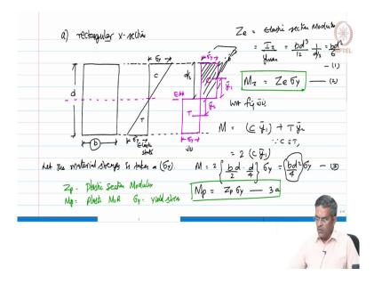
Let me write it here, I put this equal area axis. So, we can quickly find  $Z_e$ , which is the elastic section modulus which can be given by the moment of inertia about the Z axis by the distance of extreme fiber.
