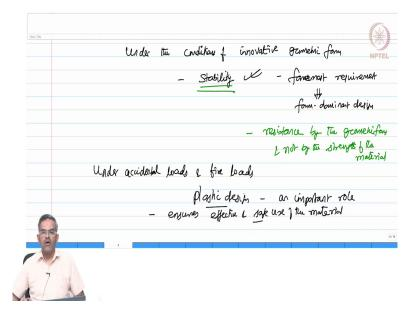
So, when we talk about an innovative geometric form, under the conditions of innovative geometric form. The foremost requirement for a structural system to function properly is its stability. So, stability becomes the foremost requirement. This is much more important when you talk about structural systems, where form dominant design is invoked.
