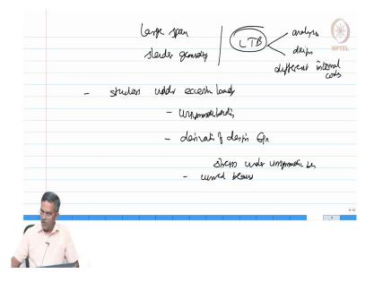
When we talk about a large span and slender geometry, then we have to also consider lateral torsional buckling. So, this course will help you to understand the lateral torsional buckling analysis and design. We will also do a design example using different international codes including Indian code for members under lateral torsional buckling in this course.
