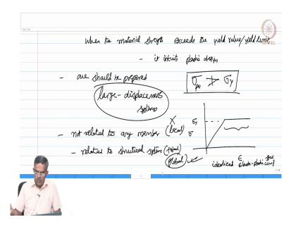
Friends, to make it very simple, when the material strength exceeds the yield value or the yield limit, then it intuits plastic design. Though in plastic design, the permissible stress cannot exceed the yield value. So, we can stress the material only up to the yield; but looking at the modified elastoplastic curve is an idealized elastoplastic curve of steel. Beyond yield, we allow large inelastic displacement.
