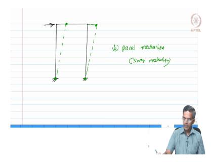
Suppose, if you have a frame subjected to a lateral load like this the frame can sway and there can be hinges formed here, here, here and here. this is called a panel mechanism, some literature advises this as sway mechanism.
