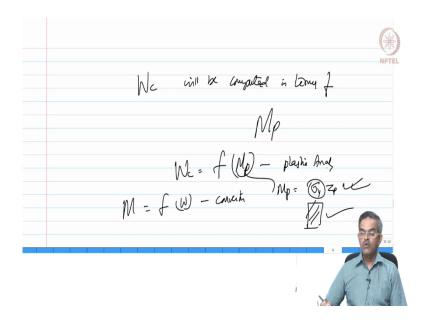
In terms of W c will be computed in terms of M p, very interesting in conventional analysis M is a function of load know this is conventional. In plastic analysis W c is a function of M p, because M p is known to me which is known independent of load it's a section property it of course, depends on material it's the section property. So, that is the beauty what we have learnt so, far in this lecture.
