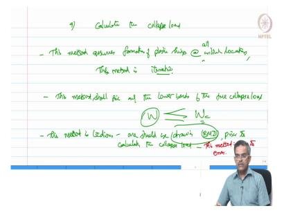
Then once you do this in the last step calculate the collapse load. Since we say this method assumes formation of plastic hinges at all critical locations this method is iterative. Further, this method shall give only the lower bounds of the true collapse load, W will be either equal to or lesser than W c what we get from the static theorem is W.
