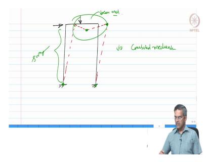
Suppose, if you have a frame which is having a combination of loads like it has got a lateral load and the gravity load then the deformation of the structure could be as marked now where the hinges can form here, here, here either here or here. So, this is called a combined
