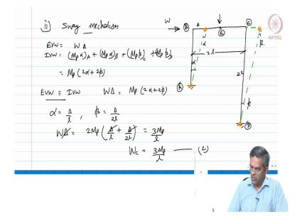
Let us go for the next one which is going to be a sway mechanism. So, the frame is going to sway to the right this point is A, B, C, D and somewhere it is E there is a load here and now there is a lateral load here W. If I call this as  $\Delta$  and this as  $\alpha$  this is also going to be  $\alpha$  and this is  $\beta$  this is going to be  $\beta$  and we know this is 2/this is also 2/.
