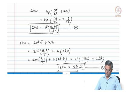
So, now I can say internal virtual work is Mp\* $(3\Delta/2/) + 2 \alpha$  which is Mp \* $(3\Delta/2/ + 2\Delta/2/)$  which is Mp \* $5\Delta/2/$ , equation number 4. I have modified the internal virtual work in a simplified form. Look at the external virtual work there are two variables, but we know they are connected to each other.
