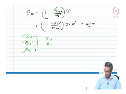
So, can you now find what is the depth of elastic core at 1.67? How do you do that? It is 1 minus M at 1.67 by Mp\*3  $h^{2}$ , h is the depth of the section. So, it will be 1 minus M at 1.67 is  $1.95*10^{3}$  you can see here  $1.95 \times 10^{3}$  by Mp is  $2.9 \times 10^{3}$  3  $h^{2}$  which is  $450^{2}$ . So, I can find very easily this will be 450mm which is completely elastic at 1.67, see here at this section it is fully elastic is it not?
