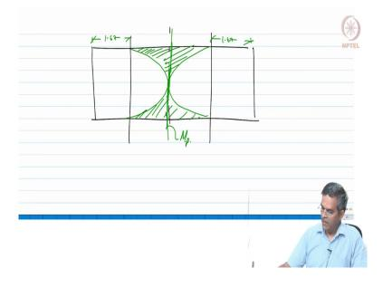
So, if you try to plot that the plot will look like this if this is my depth of the section if this is the center and this is 1.67. So, it is 1.67 from here and it is 1.67 from here and you see the hinge formation will be like this. So, this is how it is plasticized and at the mid span it is fully plastic it is Mp.
