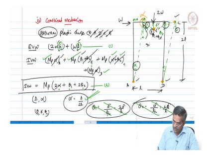
We started doing this and we said that the hinges will form at A, E, C and D it is an assumption, the hinges will form at A, D, C it is an assumption we are assuming this. The
