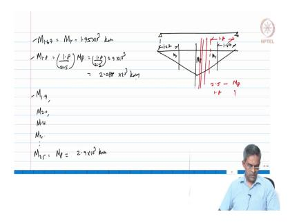
So, now let us say this is my beam in a deflected profile is the bending moment diagram as well this, this is Mp here, this is My here and this distance is 1.67 is also 1.67 by symmetry. So, I can say M at 1.67 is My which is  $1.95*10^3$ kNm. Can I find M at 1.8 from the similar triangle principle? Which will be (1.8/2.5)Mp.
