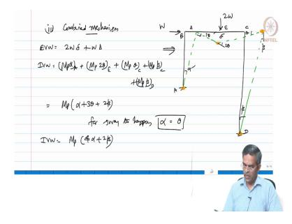
In the first iteration we got 2 Mp // now, we have 3 Mp // let us also do a combined mechanism; Let us say this is my combined mechanism I am going to assume hinges at this place and this place here and here. Let us say this is  $\alpha$  and this is  $\theta$ , this is 2  $\theta$  because this is also  $\theta$  and this is  $\beta$  and this is  $\beta$ .
