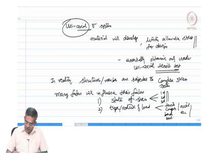
When we talk about an uniaxial stress, system the material will develop, limiting allowable stress for design. All codes look into the stress strain curve of the material, fix certain limits and say that is my design stress, is it not. Take for example, IS 800, IS 456 the steel and concrete design codes, they look into the stress strain curve of the material and fix up the value as a design stress.
