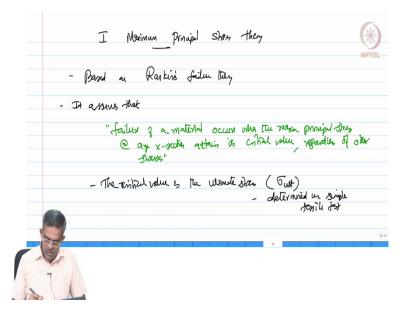
So, let us see the first one is a maximum principal stress theory, this theory is based on Rankine's failure theory, it assumes that failure of a material occurs when the maximum principal stress at any cross section attains its critical value regardless of other stresses.
