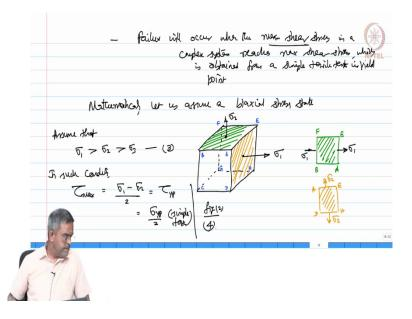
3. Failure will occur when the maximum shear stress, see the deviation. In a complex system reaches the maximum shear stress value, which is obtained from a simple tensile test in yield point. Mathematically, let us assume a bi-axial system or bi-axial stress state, the bi axial stress state is plotted. Let us hatch the surfaces, we call this stress  $\sigma$ 1, we call this stress as  $\sigma$ 2, let us say figure 2. Let us name the plane A, B, C, D, E, F, G, H.
