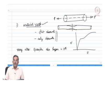
So, for example, when you take a circular bar, subject it to axial pull p the bar elongates and the diameter gets shortened and there is a neck formation and the member fails. This is a usual observation what we have seen and learned, in simple tension test in undergrad levels. So, if this material happens to be steel and try to plot the stress strain curve of this a typical stress strain curve of steel will look like this.
