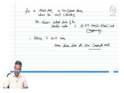
For a tensile test, in case of pure shear, where the maximum shear is developed the shear elastic limit of the ductile material is taken as about 0.57 of the tensile elastic limit. This is by experimental observations. Hence in such cases maximum shear stress theory gives conservative results.
