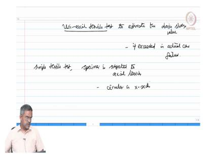
So, if you use an uniaxial tensile test, to estimate the design stress value and if this design stress value is exceeded in the actual case then we call this as a structural failure that is right. So, all the time we try to fix up the threshold limit of the stress of the material based upon uniaxial tensile test.
