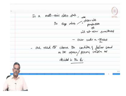
So, therefore, in a multi axial stress state the engineering values, like maximum shear stress, a principal stress etcetera will not occur simultaneously. So, they occur under a sequence and that sequence governs the failure criteria. So, therefore, one need to choose the conditions for failure based on the sequence or the governing criteria as decided by the engineer.
