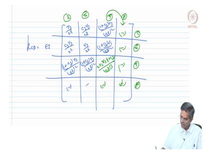
So, k CD EI times of which will be r 3 by 2l, c 3 r 3 by 2l 1 + c 3 of r 3 by 2l the whole square negative and this value will be 2 times of t 3 r 3 1 + c 3 by 2l the whole cube negative so, negative + of this column. So, the labels are going to be 2, 6, 9, 8 you can see here 2, 6, 9.
