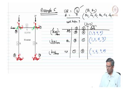
Let us do one more problem, example  $\phi$  you can now see a single way single storey frame on the screen. So, I can quickly write some inferences, the unrestrained degrees of this problem are 2, which are theta 1 and theta 2 and the restrained degrees of this problem are 3, 4, 5, 6, 7, 8 and 9.
