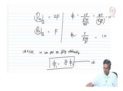
So, if I say P critical of the 1st member ok look at this figure. For the 1st member this is 2P, for the 2nd member this is P, is it not. So, 1st member this is 2P and for the 2nd member ok, let us I think use square brackets ok which will be P. So, by this logic  $\phi$ 1 should be 2P, because  $\phi$  is the ratio between the applied load and the Euler's critical load which is pi square EI by l square.
