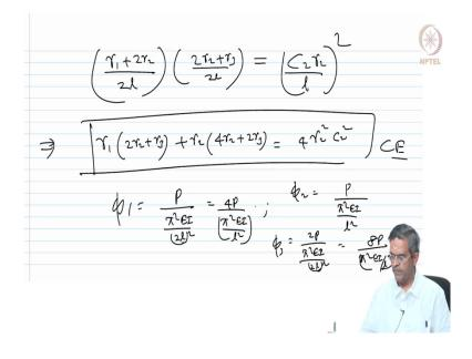
So, I can write that that is going to be r 1 + 2 r 2 by 2l see here, r 1 + 2 r 2 by 2l into 2 r 2 + r 3 by 2l should be equal to I can say should be equal to c 2 r 2 by l the whole square right, c 2 r 2 by l the whole square. So, this gives me rise to the characteristic equation which will be r 1 times of 2 r 2 + r 3 + r 2 times of 4 r 2 + 2 r 3 should be equal to 4 r 2 square c 2 square, that is my characteristic equation which I will use in MATLAB now and do it.
