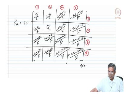
So, let us do it for the member k 2 which is again EI times of again a 4 by 4 matrix. So, this is going to be r 2 by l, because you see the length of the member 2 is only l. The length of the member 2 is only l. So, r 2 by l, then c 2 r 2 by l, 1 + c 2 of r 2 by l square.
