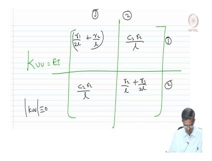
So, we have all the 3 matrices, I can assemble them and get k uu which will be E times of ok substituting we will get this as kuu. So, let us say for example, I should ok, should 1, 3, 9 and 5. So, I am looking for one more. So, I should get this and this. So, r 1 by 2l + r 2 by l = r 2
