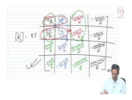
Before that let us revise quickly, that my stiffness matrix of the member is given by; the stiffness matrix is given by the basic equation which we should remember like that of a beam, which is a 4 by 4 matrix, which is ri by li, this is ci ri by li and these two by li will be this.
