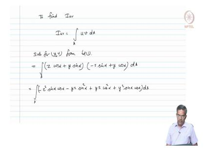
Let us also find out the cross product which is  $I_{uv}$ . We know  $I_{uv}$  is given by integral u v dA over the area A. So, we already have the values for u and v; let us see here in equation. We have equation 1, we have u and v. So, let me write it here. So, substitute for u and v from equation 1.
