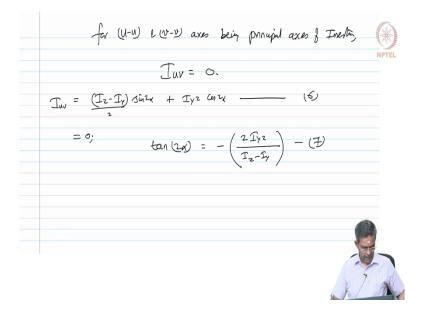
$I_{uv} = 0;$  $I_{uv} = \frac{(I_z - I_y)}{2} \sin \sin 2\alpha + I_{yz} \cos \cos 2\alpha$  $\tan \tan (2\alpha) = -\left(\frac{2I_{yz}}{I_z - I_y}\right)$
