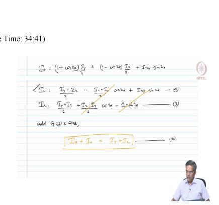
$I_{v} = (1 + \cos \cos 2\alpha) \frac{I_{y}}{2} + (1 - \cos \cos 2\alpha) \frac{I_{z}}{2} + I_{zy} \sin \sin 2\alpha$  $I_{v} = \frac{I_{y}+I_{z}}{2} - \frac{I_{z}-I_{y}}{2}\cos\cos 2\alpha + I_{ZY}\sin\sin 2\alpha$  $I_u = \frac{I_y + I_z}{2} + \frac{I_z - I_y}{2} \cos \cos 2\alpha - I_{yz} \sin \sin 2\alpha$  $I_u + I_v = I_y + I_z$
