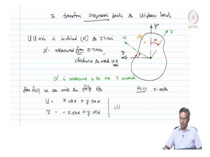
Let us look into that. So, the objective is now to transform unsymmetric bending problem to uni-planar bending that is objective now. Let us take a cross-section. Let us mark these two axes as z and y; x is normal to the screen. Let us also mark two more additional axis which is called the v and u axis.
