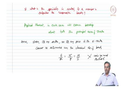
Now, the question comes what is a specialty in analysis if a member is subjected to unsymmetric bending. The answer is the applied moment, in such cases will cause bending about both the principal axes of inertia. Therefore, stress at any section or at any point in the cross section cannot be determined using the classical theory of bending that
