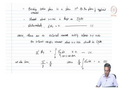
Having said this, we can now write a condition saying bending takes place in a plane parallel to the plane of applied moment.
