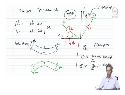
Let us say give me y axis and we mark this as my z axis, an axis here I mark this as my u-axis, this as my v-axis and we know that this angle is  $\alpha$  measured from the positive z to positive u this is. So, this is my first quadrant remember that positive y positive z. So, it is the first quadrant.
