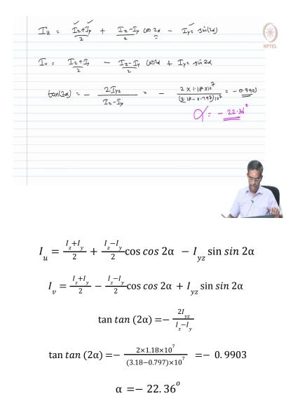
So, what does it mean, when I say  $\alpha$  is negative what does it mean? Measured clockwise from positive z axis towards positive view that is what it is.
