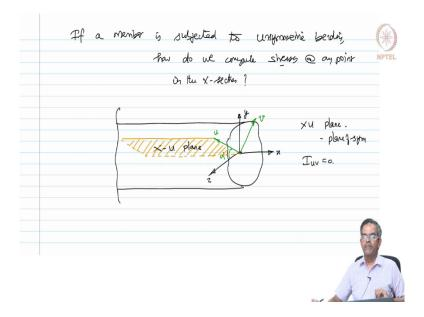
If a member is subjected to unsymmetric bending, how do we compute stresses at any point in the cross section because we said that the classical bending equation cannot be used to find out the stresses. So, how do we get this? So, let us explain this with a figure let us say I have a cross section which is arbitrary whose area is no, let us say this is my y axis and this remains as z axis and x is normal.
