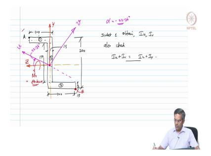
Let me mark the u-u and v-v axis and we know this angle is 22.36 degrees. So, we have marked this angle which we obtained it is always measured from positive z towards positive u that is what you have got. So, now, we know  $\alpha$  is minus 22.36 degrees let us substitute that and get  $I_u$  and  $I_v$ . So, substitute and obtain  $I_u$ ,  $I_v$  also. Check,  $I_u + I_v = I_z + I_y$ . you should check this.
