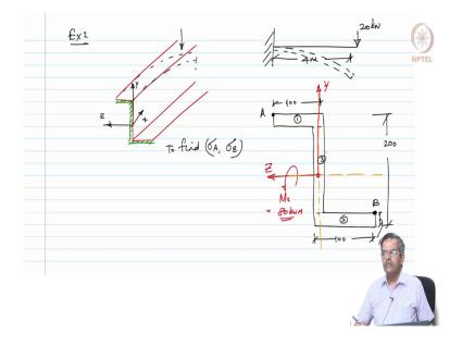
Let us do one more problem let us do one more problem which is example 2 here we take a cantilever beam subjected to a load of 20 kN for a span of 4 meters. So, the beam is going to bend this way. So, let us mark the axis, let us say this is my y-axis, this is my z-axis and this becomes my x-axis let me draw the section.
