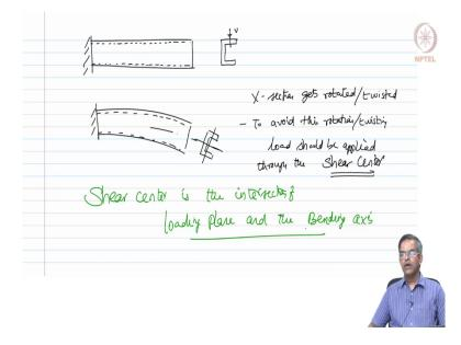
Now, let us take a cantilever beam. Let me draw the flange thickness. Let us say the section is a channel subjected to some load v. The cantilever will start deflecting under this load, where the cross section will also have this effect. So, what we say here is? Cross section gets rotated or we can say gets twisted. Now, to avoid this load should be applied through the shear center. Therefore, friends shear center is the intersection of loading plane and the bending axis.
