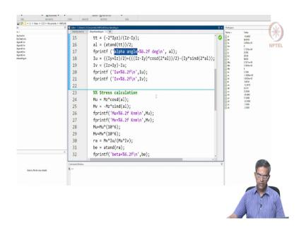
So, friends what you see on the screen is the MATLAB program to compute unsymmetrical building I section that is what we are doing. So, let us enter the values of y y as 2.579  $I_z$  and  $I_{yz}$ , which are all taken from the lecture and  $M_z$  is 4. We already have in kilo newton meter.
