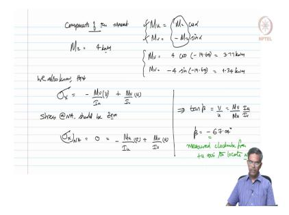
Now, having said this let us compute the components of the moment. So, now, we want to compute the components of the moment. We know the  $M_z$  value from the equation you know  $M_z$  value will be 2 into 2, which is 4 kNm. Which will cause bending this way. So, tension at the bottom compresses the top.
