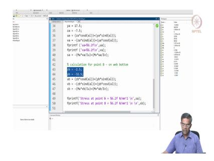
Then it computes  $M_u$  and  $M_v$  then we have to enter the coordinates for the point A and coordinates for the point B. Please see that. Once we enter the program runs. I will get the stress at point A and point B. Let us run this program. So, the program is run.
