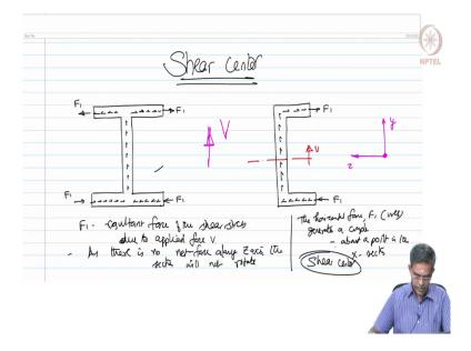
Now, let us start discussing something on shear center. So, we will does something about shear center to understand shear center. Let us first see the internal force distribution in a given section. Let us take for example, an I section. And a channel section whatever may be the dimension.
