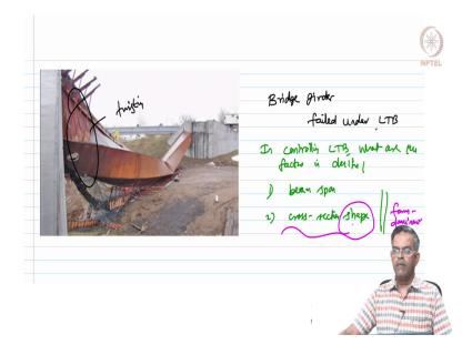
This is a photograph of a bridge girder failure under LTB. One can very well see the twisting of the cross-section and the thickness of the flange is phenomenally lesser which cannot sustain or offer enough torsional rigidity to this. So, now in controlling LTB, let us say what are the factors in the design. 1, Of course the beam span; if it is too long then it is dangerous. 2, The cross-sectional shape.
