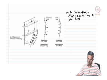
Look at figure 16. On the contrary, tension flange tends to keep the beam straight. This lateral bending of the section creates restoring forces that oppose the moment because the section tends to remain straight. These actions generate lateral forces which sometimes are not adequate to prevent the section from lateral deflection and that is what we call as resistance against lateral torsional buckling which we can see from this figure.
