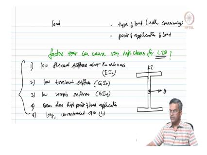
The fourth factor is a load. So, depending upon the type of load, whether it is uniform distributed load, whether it is concentrated load etcetera one can also result in lateral torsional buckling. The next is the point of application of load where the load is applied along the length of the member and along the breadth of the member. So, these factors are very useful in designing the beam to control the lateral torsional buckling and that can be avoided.
