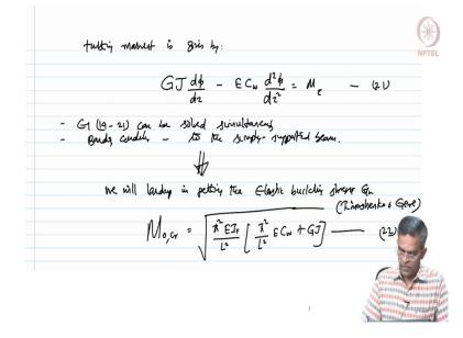
Now, the twisting moment is given by G J d  $\phi$  by dz - E C w d<sup>2</sup> $\phi$  by dz<sup>2</sup> is M $\tau$  this is equation 21. Now, we can solve all these three equations. So, equations 19 to 21 can be solved simultaneously. And, we can apply respective boundary conditions for the simply supported beam the boundary conditions will be applicable to the simply supported beam.
