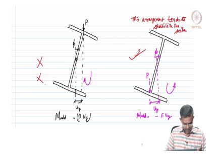
Let us say, if you have a section let us copy the same figure here. When a load is applied here, there is a line of action of the load. So, C g let us say this is U y and we call this shift as  $\phi$ . This is the load P. So, the additional moment caused in this case will be the load P into U y.
