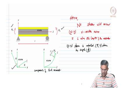
So, let us see this figure, it is subjected to uniform moments at the ends M0. under such arrangement no shear will happen. No shear will occur. So, the X-Y cross-sections cross-section axis and the Z-axis or marked as shown in the figure. So, X-Y is the cross-section axis and Z is along the length of the member. Now, let us look into the bottom figure where I am marking the components of the end moment.
