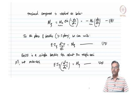
Now, the torsional component is resolved as below. Will be given by M x sin (- du/dz); as z is the axis along the length of the member which came you know said as  $- M_0$  du/dz equation number 18. So, one can very well notice here, M x replaces M0 because M0 is the end moment acting about the X-X plane. Now, in the plane of bending which is the Y-Z plane we can now write E I  $\zeta$  d<sup>2</sup>v by dz<sup>2</sup> will be M  $\zeta$  equation 19.
