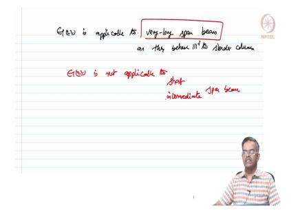
Equation 22 is applicable to very long span beams and as they behave similar to slender columns; short and intermediate span beams will not be applicable or governed by equation 22. So, we can say equation 22 is not applicable to short and intermediate span beams. So, friends, the elastic buckling strength equation which is governing the lateral torsional buckling is applicable to long span beams. Now, let us see what the mechanism behind lateral torsion is buckling as explained by Eurocode.
