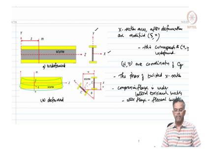
So, this is my undeformed geometry. And, the second figure what you see is the deformed geometry. So, we are considering a simply supported beam, as loaded. The cross-section axis are now modified, the cross-section axis after deformation are modified as  $\zeta$ ,  $\eta$  axis as you see in the figure and this corresponds to Z, Y axis which is undeformed,. Let us also understand that u and v are coordinates of the C g of the section which will now designate the new position after twisting.
