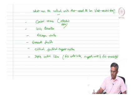
What are the critical units that need to be blast resistant design? Ask this question. What are these units? One, control rooms both electrical and mechanical. Two, living quarters where the occupancy rate is very high. Escape routes, evacuation facilities, critical structural support systems and safety critical items.
