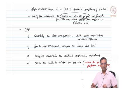
Blast resistant design is a part of structural strengthening of buildings. It is one of the measures to minimize the risk to people and facilities from hazards of accident explosions happening in the industrial units. So, the primary objective of the blast resistant design is essentially to minimize risk to people. Now, let us ask a question what are the steps involved in Blast resistant design.
