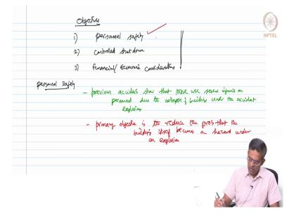
What are the objectives? The primary objective of providing blast resistant design for buildings are as follows: 1, personal safety; 2, one can initiate what is called as controlled shutdown; 3, financial or economic considerations. So, these are the three factors which control the objective of blast resistant design. Let us see one by one in detail. Let us talk about personal safety. Blast resistant design should provide a level of safety for persons inside the building.
