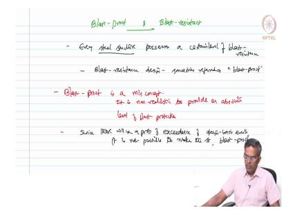
Friends, every structure which is being designed be it strategic non-strategic has some level of blast resistance, because blast resistance is a part of strengthens structural requirement and buildings constructed by steel essentially do possess this inherent characteristic. So, I can now say very clearly here every steel structure possess a certain level of blast resistance.
