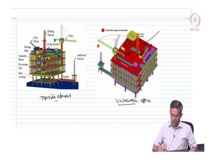
Let us talk a classical example of an offshore platform where the top side is being shown on the figure. So, this is a top side element. On this top side, the vulnerable region for impact loads is being marked. This is a vulnerable region. Let us have a model of this type.
