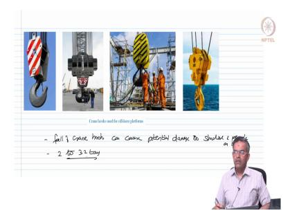
Now, the varieties of cranes being used in offshore structures are shown on the screen. So, the fall of crane hooks of these heavy mass and other objects is frequent and fall of crane hooks can cause potential damage to structure and people on board. Look at the typical crane hooks being shown on the screen. They are very massive and they vary from 2 to about 32 tons that is the range of weight these crane hooks have.
