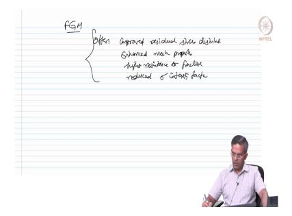
So, for our convenience let us quickly recollect that FGM offers improved residual stress distribution. It has enhanced mechanical properties. It has got higher resistance to fracture and it has got reduced stress intensity factors. So, we are not discussing about the FGM properties at this moment.
