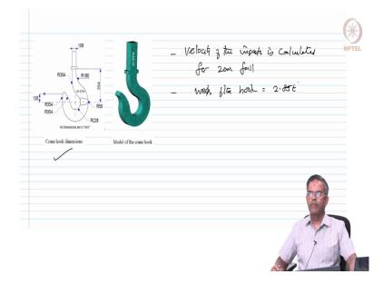
We will start directly going to the model of the crane hook. The model of the crane hook is showing on the screen whose dimensions are given here. The velocity of the impactor considered in the analysis is calculated for 20-meter fall and the weight of the hook is taken as 2.85 tons which is subjected to the CG of this hook.
