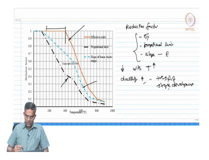
Having said this let us talk about steel property at a higher temperature. The figure what you see on the screen shows the reduction factor on different parameters of steel when the temperature is increased from about 200 degree centigrade to about 900. So, there is a reduction factor applicable to yield strength, proportionality limit and slope of the elastic range which will help you to compute the Young's modulus.
