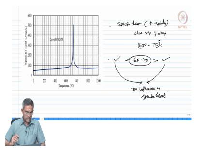
Similarly, if you look at the specific heat requirement, it gradually increases and the specific heat increases rapidly in the close range of temperature varying from 650 to about 750 degree
