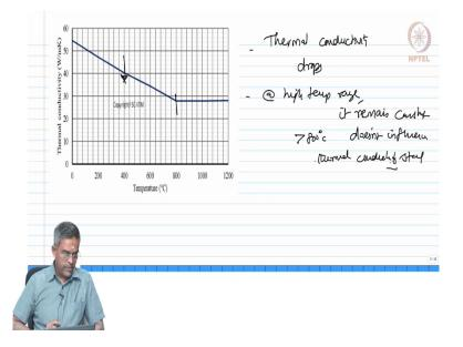
So, let us see the other properties of steel. This curve shows the variation of thermal conductivity which drops the thermal conductivity drops you can see here it drops with the increase in temperature. It is also see that up to 800 degree Celsius it drops then at higher temperature range it remains constant. So, temperature more than 800 degree centigrade approximately does not influence the thermal conductivity of steel.
