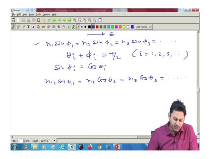
So, at every interface, I can write the Snell's law. And I can have straight wave equation n 1 sin phi 1 is equal to n 2 sin phi 2 is equal to n 3 sin phi 3 and so on. Now, from this geometry, it is easy to check that theta i plus phi i is equal to pi by 2 when i is 1, 2, 3. The layers in each
