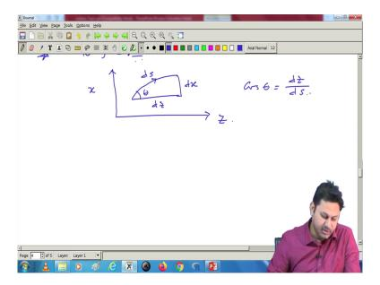
With this note, now I can derive an equation which we call the ray equation. So, I have a structure like this. This is x, this is z. And some arbitrary path, I am drawing this path is followed by the ray. This is the length I write ds, and this angle is theta. So, this is dz, and this is dx. So, the ray is suppose the ray is moving in this way.
