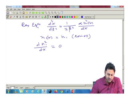
If I want to find out what happened in the core, then n 1 in x equal to n 1 which is a constant. So, definitely this value will be 0, sorry this is so I should write at n square, because this is the original equation. So, this equation this portion the right hand side is simply 0.
