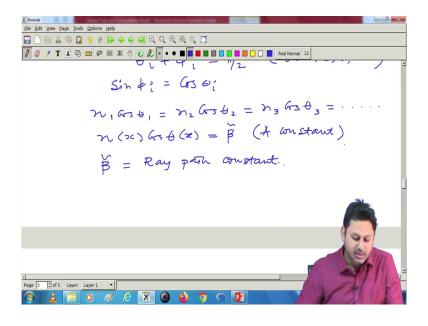
So, in general n x cos theta which is again a function of x is equal to some constant I write as beta tilde, a constant. This quantity will remain constant. So, this beta tilde is called which is a constant quantity is called the ray path constant, which is not changing whatever the ray it follows, whatever the ray I launch then for that ray, for example this arbitrary ray that is coming going from A point to B point, every every at every point over this ray beta tilde is constant.
