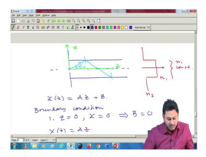
So, my expression is the ray will follow this path which is a straight line A z plus B, this is the path. And now if I put the boundary condition, so boundary condition, one boundary condition is if I look carefully to this ray, whatever the way I draw here, the boundary condition the one boundary condition is obvious that at z equal to 0, x is 0.
