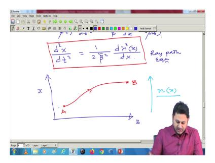
So, you should remember that what we have done earlier that this is my z-direction and this is my x-direction. And a ray is moving from this to this path suppose this is point A and some point B, ray is moving. But along this direction, we have a change of refractive index; along this direction, we have a change of refractive index n is a function of x.
