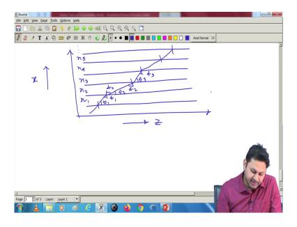
To make this calculation systematic, let us divide this refractive index profile into small parts. So, I have along this direction I have x; along this direction, I have z. And suppose the refractive index, there is a change of refractive index. And this change of refractive index, I
