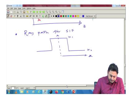
So, let us start with one profile. So, ray path for step index fiber. So, I know the refractive index profile for step index; which in the last class we mentioned, how the mathematical form will look like. We have used it earlier. So, this is n 2; this is n 1. So, n 1 and n 2 is constant here.
