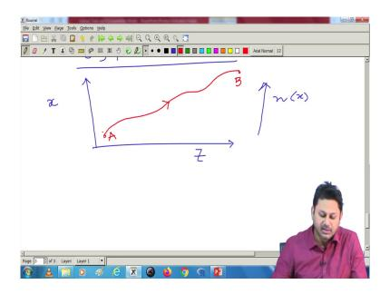
Suppose, we have a arbitrary refractive index. If we have a arbitrary refractive index over say x-direction and this is the z-direction. And along this direction, I have a change of refractive index as a function of x. If I have a change of refractive index along this direction, so what happened, if I launch a ray it can follow certain paths; depending on the value of the refractive index.
