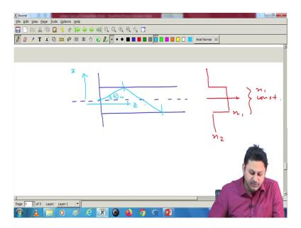
So, that means, if I have a step, step index fiber, this is the structure of the fiber or waveguide. And the index profile if I draw which is something like this. So, this is n 1, this is n 2. And in this region, n 1 constant, it is constant; there is no change in n 1. And now if I launch a light here, then it should move with the straight line. And then there is a reflection that is happening total internal reflection.
