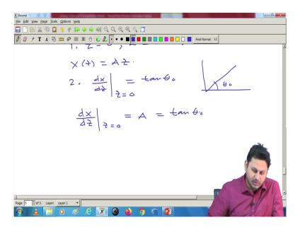
So, the boundary condition 2 gives me d x d z at z equal to 0 is tan theta 0, because initial angle is given. So, this angle is given. This is theta 0. So, the initial angle is given. An initial angle is nothing but the derivative with respect to derivative of x with respect to z at z equal to 0 point. And if I calculate that, I can find from this equation that d x d z at z equal to 0 is equal to A which is tan theta 0.
