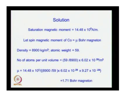
Let s assume that this spin moment is mu in bore magnetron the density is 8900. So, the number of atoms cobalt atoms per meter cube is given by atomic. Weight divided by the density times the Avogadro number and therefore, mu is from 14.48 into 10 to the power 5 divided by suppose bcc n substituting for n well into bore magnetrons and that will be 1.71.
