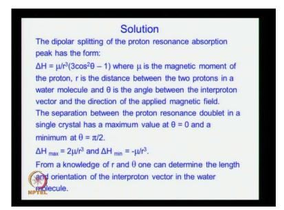
In order to answer this we have to start from dipolar splitting of the proton resonance in water, this is given by we discussed this already mu by r cube into three cause squire theta minus 1, where mu is the proton magnetic moment which is known r is the distance between protons. And theta is the angle between p p vector and the applied magnetic field. So, this means that this dipolar splitting of the photon resonance gives a doublet structure like this.
