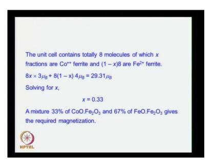
And the unit cell of the ferrite has eight molecules, therefore we have to determine the fraction x of cobalt ferrite.
