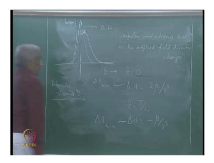
So, instead of where there is a single proton resonance speed we will have doublet structure like this somewhat like this. So, this is the separation which we call delta H. So, has one rotates the applied magnetic field the angle theta changes in therefore there will be an angular variation of this dipolar splitting as the applied magnetic field direction changes in particular in theta is 0 three cross squire in theta is three.
