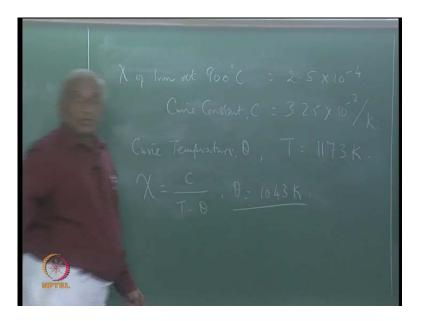
Next is a problem on the magnetic susceptibility of ion at 900 Celsius is 2.5 into 10 to the power minus 4. Here also given the curie constant c as 3.25 to 10 to the power minus 2 per k we are as to find the curie temperature for which the standard symbol is theta in the expression for the susceptibility. And we are told that the temperature is 900 Celsius
