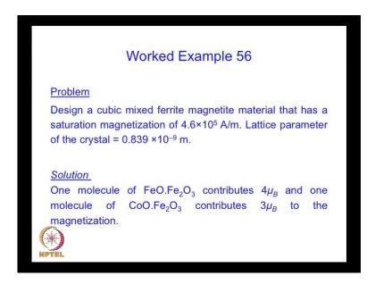
We are given the lattice parameters of the basic crystal is all eight three nine into ten to the power minus nine meters. So, basically we have the basic ferrite is magnetite in which the ion and contributes four bore magnetrons, and we mix it with cobalt right in which case the cobalt ion cobalt s ion as a magnetic moment of bore magnetron. So, we are to design a mix ferrite whose saturation magnetization is given from the value of saturation magnetization given.
