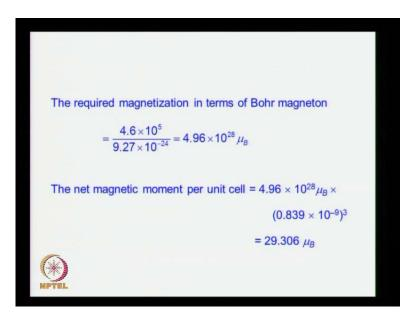
So, that would be now if we have a unit cell the net magnetic moment per unit cell is this is what we want times the volume of the unit cell the lattice parameter is given is a cubic lattice. So, it is just a cube or the lattice parameters. So, this turns out to be. So, we have to make a material which has a magnetic moment of 29.306 bore magnetrons.
