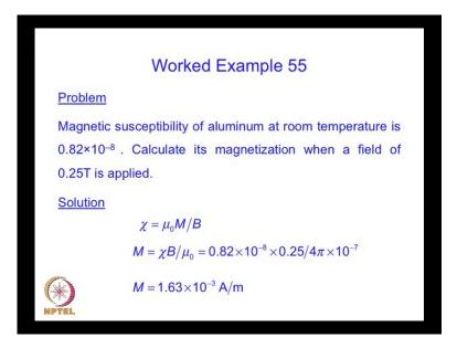
Next we are has to calculate the susceptibility of aluminum at room temperature no we are being given susceptibility at room temperature as 0.82 into 10 to the power minus eight. So, we are as to calculate its magnetization in an applied magnetic field 0.25 teals again we know the relation between the susceptibility mu naught m by b. So, the magnetization is 5 times b by mu naught. So, substituting the value is turns out we have into 10 to the power minus 3.
