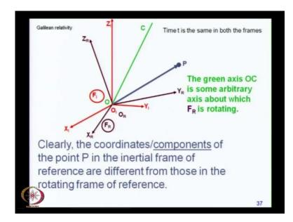
So, we consider a frame of reference F I and there is X axis, Y axis and Z axis and there is another frame of reference which will be the rotating frame of reference with the subscript R and t is equal to 0, let us say that the two frames of references are on top of each other, their origins coincide the axis are corresponding, the corresponding axis are parallel to each other. Then, at a certain instant of time one frame starts rotating with respect to the other about a certain axis.
