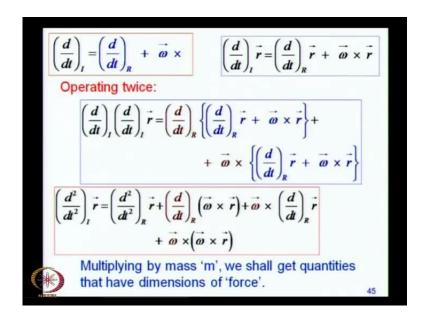
If it operates on the position vector, we get this relation that the velocity in the inertial frame of reference is equal to the velocity in the rotating frame of reference plus the cross product of the position vector with omega which is omega cross r. This is what happens when you take the first derivative.
