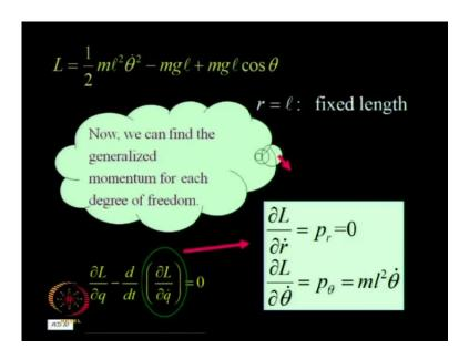
You can do the same for a simple pendulum. You have to be a little careful over here. Now, this diagram is almost self-explanatory. So, the potential energy will be given by this. If it is measured with respect to this reference point, then mg times this distance h will be the potential energy which is l times one minus cos theta; l being the length of the pendulum and we presume that this length is not changing; it is not elastic; it is rigid. So, you have got the potential.
