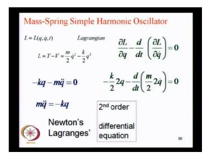
So, if you take a mass spring oscillator, the first thing to do is to set up the Lagrangian which is T minus V. So, the kinetic energy is half q dot square times the inertia. So, m by 2 q dot square minus the potential energy which is k by 2 q square; k is the famous spring constant. So, you have set up the Lagrangian.
