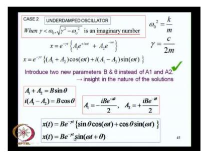
So, you can write these exponential functions in terms of the cosine and the sine functions. This is the nice way of looking at it; because when you write it as such - you find that you, can transform this form in which you have written the same solutions in terms of the cosine and the sine functions. By introducing two parameters B and theta instead of A 1 and A 2. As long as, we do not introduce additional parameters.
