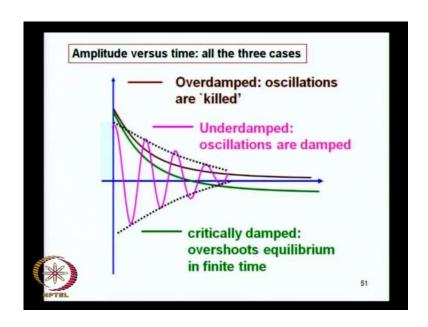
So, the next attainment of equilibrium will be only after infinite time; so, these are the various cases to put them all together. These are the various profiles that you see if you plot amplitude as a function of time for all the three cases. So, you have got the over damped oscillator which really would approach equilibrium point only as t goes to infinity.
