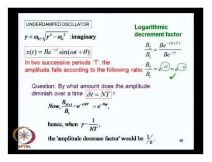
So, this is the factor through which the amplitude falls over successive periods and you know the amplitude decrease factor would be 1 over e because if you let gamma equal to 1 over NT if gamma is equal to 1 over NT then this successive ratio it will go as 1 over e. So this is the factor.
