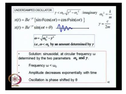
So, here you see that this amplitude of this oscillatory motion diminishes and if you look at the envelope envelope it will go down exponentially. So, this is the general function this is oscillatory it oscillates at a frequency omega which is determined by omega 0 and gamma.
