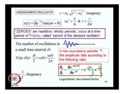
So, this is called as under damped oscillator because motion is damped but it is not damped the way the over damped oscillation was so as oppose to this. This is called as under damped oscillator.
