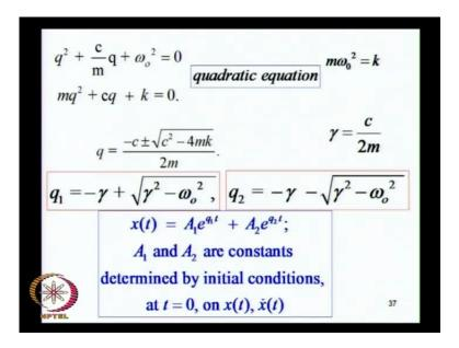
From differential calculus, we have reduced the problem to algebra. Iinstead of dealing with a first order derivative and a second order derivative and having a second order differential equation, all we have to do is a quadratic equation in q which we know how to solve. It has got two roots.
