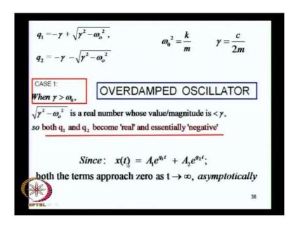
So, we will now consider the case when gamma is greater than omega 0. This case gives us a damped oscillator which is in fact, called as an over damped oscillator and I will explain why it is called as an over damped oscillator.
