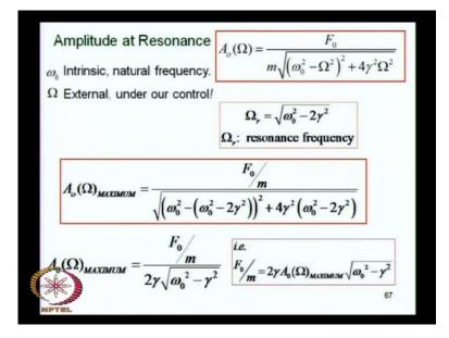
Now, what is the value at the resonance frequency? What is the value of the amplitude at the resonance frequency? We already know that the amplitude changes with frequency. We are now asking what will be this value when the frequency of the driving force omega is equal to the resonance frequency. So, all you have to do is to substitute this factor omega by the expression for the resonance frequency and you get the expression for the maximum amplitude.
