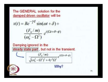
The other part which is the solution to the homogeneous equation is the transient part because it is going to die out in a finite amount of time. It hass got the a diminishing amplitude of the under damped oscillator. It is going to die out in a certain amount of time. So, that is the transient solution.
