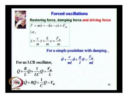
So, we will setup an equation of motion in which the net mass time acceleration for the object which is mx double dot for a one dimensional oscillator is equal to the restoring force which is minus kx. Then there is a damping term which is minus cx dot; this is the term that we discussed yesterday. In addition, there is a driving force F dr. So, your equation of motion is this: F mx double dot is equal to minus kx minus cx dot plus F, driving force.
