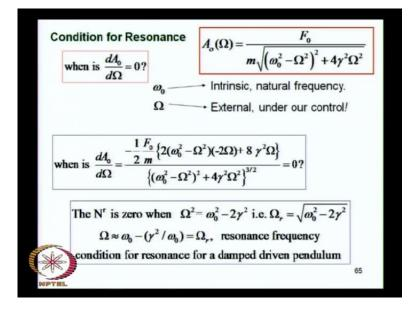
So, anyhow, the condition for resonance which is when we are going to have the maximum amplitude is dA by d omega equal to 0. So, this is where you take the derivative of the right hand side with respect to omega. So, you just do it carefully because you have got a denominator, omega appears in the denominator and that too twice; once over here and once over here (Refer Slide Time: 28:48).
