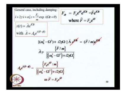
So, here you go. You now have this form of the driving force and in this differential equation; you substitute for x dot and x double dot that you have already found over here and you get an algebraic equation. Then, we have to solve this algebraic equation so that we can understand what is the nature of the solutions.
