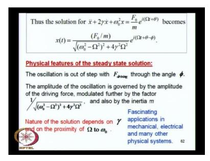
This is the solution for the differential equation. This is a steady state solution. In addition to this, there will be another solution; I will get to that.
