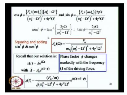
So, it is this damping which is responsible for the phase lag between the response of the damped oscillator to the periodic oscillations. If gamma was 0, this would go to 0. So, it is because of this damping that there is an additional phase that steps into your analysis.
