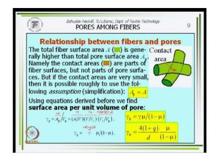
So, we derived equations which are valid for pores for our air fibers; we can say air tubes. These equations, these equations give together different quantities, different quantities s p, d p, V p, A p, q p, gamma p which are valid for pores. Nevertheless, we usually need, we do not know these characteristics. We know the characteristic of fibers, we know fiber diameter because we know fiber fineness, we know fiber surface and so on and so on.
