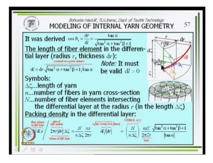
Earlier, we derived cosines of angle theta i, angle theta i, this green angle between the vertical direction of yarn axis and the right element of fiber. Is it not? We derived it. So, it is defined d r by d l; it was shown and we derived that it is tangent alpha by square root of tangent square alpha plus tangent square beta plus one.
