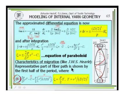
So, we obtain finally this relation. What is this equation? For a parabolic zeta and radius, on which is laying the trajectory of fiber. This parabolic, this approximation equation used by Professor Hearle; Hearle maybe is here and he must be very old man. I was a little boy and he was a top man of yarn structure in my young years. He was a professor on UMAST, Manchester, on the university Manchester, and author of lot of special models.
