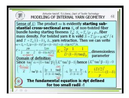
What is the sign of our parameter K in this fundamental equation? It is derived here, the product and times as is evidently starting substantial cross sectional area; substantial cross sectional area S 0. For a fiber bundle, cross sectional area of all fibers, its n times cross sectional area per one fiber and in per one fiber bundle it is S. So, that S 0 is T 0, starting fineness of per one fiber starting from which we create the yarn by rho; rho is fiber mass density as every times.
