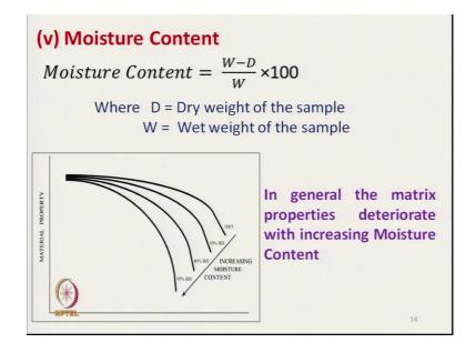
So, we must know the moisture content of matrix material because this moisture content affect the characteristics of matrix. So, this picture we can see that as the moisture content increases this is the dry 50 % relative humidity and this is the 95 % relative humidity, as the relative humidity increases, so, increase in moisture content is there. So, drop in characteristics is there. So, it is a; there is a sharp drop in the material property.
