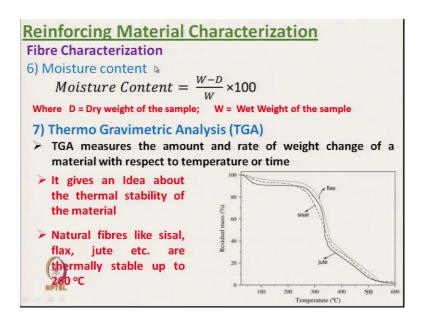
So, moisture content we can measure by measuring the dry weight of the sample and wet weight of the sample. So, we take the material and we first condition the material at standard temperature and humidity. And after that we take the W, which is wet weight of the material.
