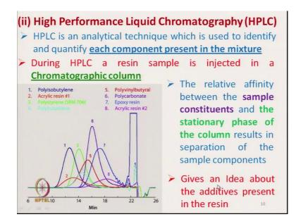
Next is that HPLC; High Performance Liquid Chromatography. So, what is this; HPLC is an analytical technique which is used to identify and quantify each component present in the mixture. So, the matrix material may be of mixture of different components ok. And this will show, this will quantify each components ok. During HPLC a resin sample is injected in a chromatographic column there will be a chromatographic column. And resin sample will be injected.
