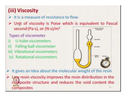
Next is the viscosity; which is extremely important characteristics of any matrix material. So, as I have mentioned at low temperature the thermoset matrix has got advantage of very low viscosity. Low viscosity means the flow through the pores of the fiber penetration of matrix material will be easy. On the other hand the thermoplastic matrix in normal temperature they are solid like polypropylene. To reduce the viscosity we have to increase the temperature.
