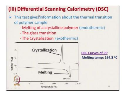
So, this test gives information about the thermal transition of polymer sample. So, thermal transition means here at certain point it will actually absorb heat or it will release heat. So, the during the melting during melting it will it is a endothermic reaction. That is the heat it will take the heat melting ok. And during crystallization which is exothermic so it will release heat. And also you can measure the glass transition temperature.
