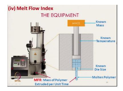
So, this is the equipment where the molten polymer is actually of known mass is placed here. And temperature is maintained we know the temperature at what temperature we have to keep the material this molten polymer and the die is kept here at the bottom and when the polymer molten polymer is flown through the die the quantity required quantity per unit time it is measured the mass of polymer extruded per unit time it is measured and that shows the melt flow index.
