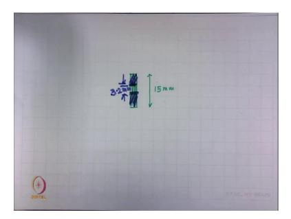
So, this is the way which goes. This is the fiber bundle this length is 15 millimeter. And once we are gripping these are the grips this is the jaw and here it is a jaw and this length this is gauze length which is 3.2 millimeter. So, bundle strength test is done in this fashion. And in addition to the bundle strength we can also perform the single fiber strength test. And the gauze length here it is 25 mm for manmade fiber and 10 mm for natural fiber ok.
