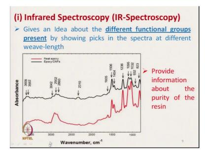
So, what is IR spectroscopy? It gives an idea about the different functional groups present by showing the peaks in the spectra at different wavelength. So, in x axis it is a different wavelength and the spectra at different wavelength and y axis it shows the absorbance. So, for different functional groups present in the material it shows by the peaks these are the different peaks.
