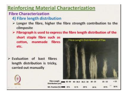
Now, the fiber length distribution is also an important characteristics, longer the fiber higher the fiber length contribution to the composite. And for cotton we can use fibrograph which actually measures the fiber length distribution ok, of the short fiber. In addition to cotton we can also use the manmade fibers. But as far as bast fibers are concern like jute fiber or flax ok.
