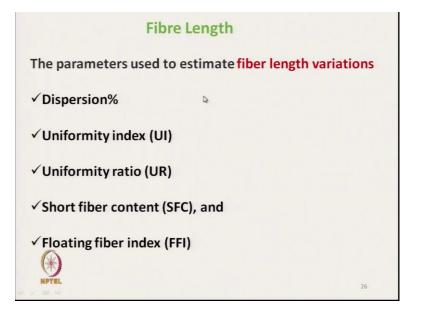
And the parameters used to estimate fiber length distribution or fiber length variation; these are dispersion percent, uniformity index, uniformity ratio, short fiber content and the floating fiber index. So, these are the different characteristics which shows the dispersion characteristics of fiber. Again all these terms you can actually learn in other course which is a textile testing course or evaluation of textile material course.
