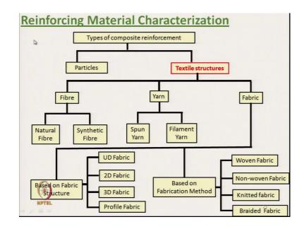
So, these are the reinforcing material. First is that particles which we will not discuss because we will be discussing the textile structure. So, textile structure these are of basically three types; one is fiber, yarn and fabric. Fiber natural fiber and synthetic fiber, yarn spun yarn or filament yarn and fabrics are first is that based on the fabric structure Unidirectional fabric 2D dimensional fabric 3D dimensional fabric and profile fabric.
