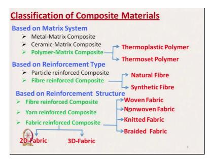
So, composite materials are classified based on matrix system based on reinforcement type and based on reinforcement structure, first based on matrix system. So, the matrix which is used in composite are basically of three types; first is metal matrix composite, next is ceramic matrix composite and third one is polymer matrix composite. In our discussion we will concentrate on evaluation of polymer matrix composite materials.
