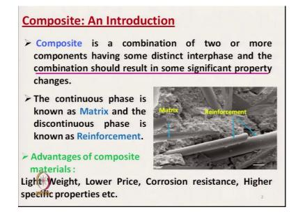
So, composite is a combination of two or more components having some distinct interface and the combination should result some significant property change. So, there must be some significant improvement in properties. So, that is why we prepare composite the composite has got three distinct components. One is matrix component, second one is reinforcing component and third is that distinct interface. So, combination should result significant improvement in characteristics of material.
