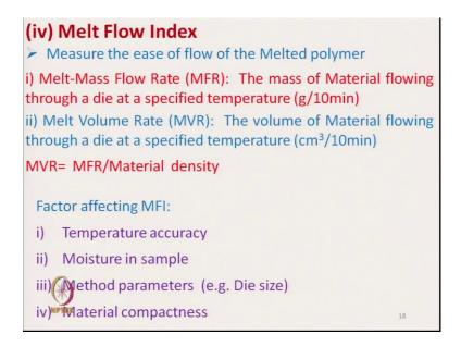
So, if the melt flow index, the flow characteristics is better it is a good in a particular temperature. Then the composite will be better characteristics will be better. It measures the ease of flow of the melted polymer. So, how easily the polymer melt flows inside the structure. Melt mass flow rate the MFR it is called MFR. The mass of material flowing through a die of specific dimension at a specified temperature.
