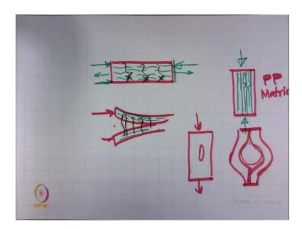
Suppose, this is a composite material, and fibres are aligned in this direction. And what is in-plane force, this is the in-plane. Here we are talking about out of plane stress. So,
