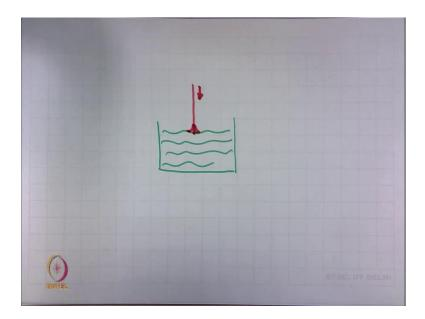
Like this is measured the surface energy or contact angle is measured by this method. There is a liquid; liquid of known surface free energy. And once the fibre is dipped and it will actually try to the liquid will try to rise and it will form a contact angle, and that will have some downward force. The liquid contact with the fibre, will start pulling the fibre downward and that force is measured.
