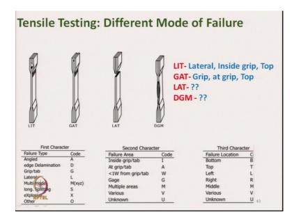
So, this is showing the composite specimen with tab portion. And <u>this-these</u> modes are expressed with the three letters ok; tensile failures are expressed with three letters. The first character which is one single letter character, which is showing the failure type, it is a type of failure. Second character which shows the area of failure area which at which area the failure takes place<del>.</del> <u>a</u>And third character is the location of the failure.
