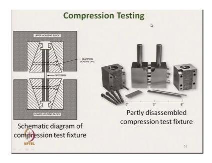
This is the compressive testing fixture where this is a specimen. And this specimen is gripped by two fixtures with the help of screw. And then they are compressed along the plane ok, not across the plane, and the compressive stress is calculated ok. These are the partly disassembled compression test fixture, so that we can use for testing.
