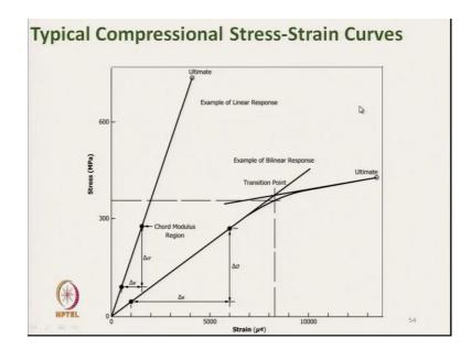
Here again it is a ultimate compressive stress here. And so this is a linear response. There may be some non-linear responses are there, and they are actually calculated in similar way the to that of our tensile stress which we have already discussed. And the failure mechanisms, type of failures can be expressed in the similar way as we have discussed earlier also.
