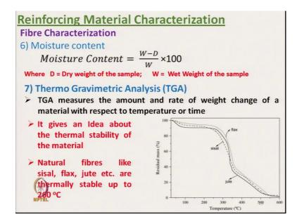
And TGA measures the amount and rate of mass change of a material with respect to temperature or time. And this curve shows that the residual mass that is change of mass in case of flax, jute, sisal occurs around a temperature around  $260^{\circ}$ C, so that means, the materials are stable up to  $260^{\circ}$ C.
