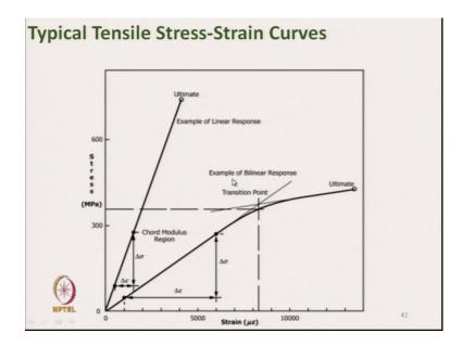
Now, this is the typical curve ok, where in x-axis it shows the strain; and in y-axis it showing the stress in MPa. This is one curve for a particular composite, where this point, it is a ultimate stress, ultimate point. This is the ultimate strain from there you can calculate an ultimate stress we can calculate. And this is showing the linear response of the composite. Before it bent, it reaches the ultimate point ok.
