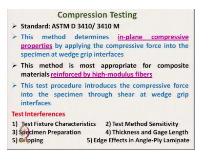
Next method is the compression testing. This method determines in-plane compressive properties by applying a compressive force into the specimen at wedge grip interface.
