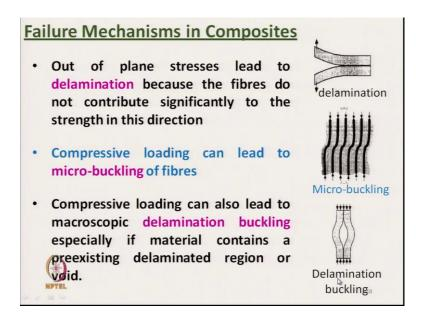
Out of plane stress leads to delamination because the fibres do not contribute significantly to the strength in this direction. Now, this is the picture. Now, let us see.
