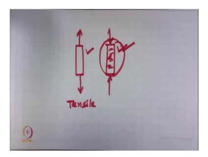
Like what we have discussed till now it is a tensile tensile characteristics, and we can measure the tensile stress, tensile modulus. But there are many applications where composite undergoes the compressive load, not the tensile load. So, tensile load is important, but compressive load in composite is also very important. And due to the compressive load, there will be a failure in composite structure and which we must
