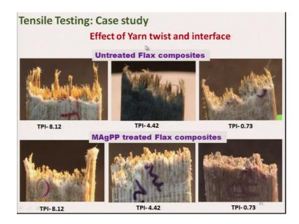
Now, few experimental data, the effect of yarn twist and interface. So, we have made some interface with MAgPP treatment on flax fibre. So, untreated flax fibre composite, after tensile breakage, these are the photographs. And here we have studied the effect of twist and interface. So, if we see the left side this picture, it is untreated flax composite with the with high twist 8.12 twist per inch. And twist is gradually , reduced and right side it is a TPI is 0.73.
