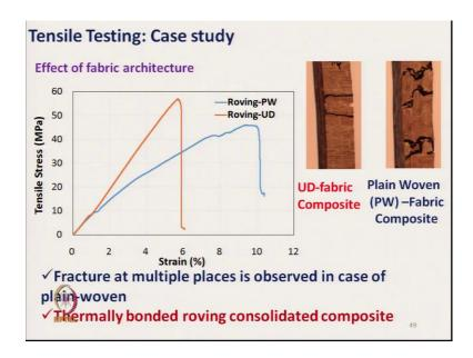
Another case studies you can see here the roving material effect of fabric architecture. So, one is that UD, roving-UD means unidirectional fabric composite. So, fabrics are made of the unidirectional orientation of roving. Another construction is that plain woven PW fabric composite, so that is that-one is the roving UD and roving PW. Here we can see clearly the roving-UD results higher tensile stress than roving-PW that is the woven fabric, whereas the roving PW results higher strain.
