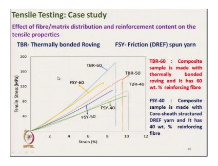
So, if we compare <u>this\_these</u> tensile characteristics with thermally bonded roving and friction spun yarn for different proportion of reinforcing fibre like TBR-60 which indicates the composite sample is made with thermally bonded roving. And it has the weight percent of 60 percent reinforcing fibre, FSY-40 which means composite sample is made with core sheath structure of DREF yarn, and it has 40 percent reinforcing fibre.
