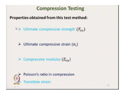
And the properties, which we get from the compression testing is the ultimate compressive strength, ultimate compressive strain, compressive modulus Poisson's ratio in compression, and transition strain. So, during compression, we will get almost similar type of stress-strain curve.
