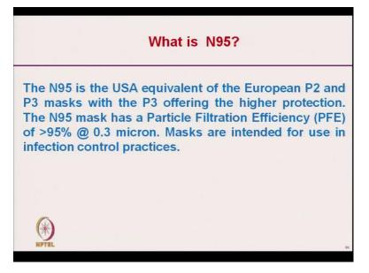
And another term which is used for mask is N95, it is very commonly used. It is the US standard which is equivalent European standard is P2 and P3 masks with the P3 offering higher protection. The N95 mask has a particle filter efficiency more than 95 percent with the particle size of 0.3 micron. So, N95 is showing that if we use 0.3 micron particles, it will have efficiency more than 95 percent. So, these masks are intended for use in infection control practices. We will stop here.
