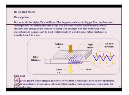
So, it is suitable for high efficiency filtration. Pleating process leads to bigger filter surface and consequently the smaller pressure drop. So, this will result lower pressure drop. And the end uses are the pre-filters, HEPA filter used for air ventilation and air conditioning system, auto cabin air filter. There are different industrial applications are also there. So, this is used and even it is used for the automobile filter.
