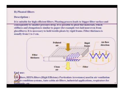
Another filter is it is called pleated filter. Pleated filters are basically it is a variation of the flat filter.
