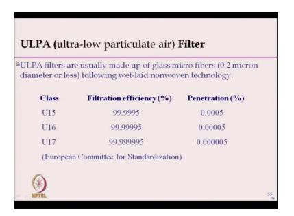
But, if we want higher filtration efficiency than this we have to go to ULPA filter, it is in the same series, but for high filtration efficiency ultra-low particulate air filter, where the filtration efficiency is very high. So, U 15, U 16, U 17, U 15 -99.9995 ok. And U 17 is almost 100 percent, the arrestance percent is very very penetration is very very low, here where arrestance is very high. So, if we need very high filtration efficiency, we must use U 17 type filter.
