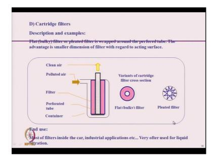
Next type of filter based on the shape is the cartridge, filter cartridge is very commonly used for many applications like liquid filter or even air filter ok. This is the filter cartridge, where the flat that is bulk filter or this is the flat filter or pleated filter is wrapped around a perforated tube. This is the perforated tube, this flat filter or pleated filter is wrapped around this, the advantage is that smaller dimension of filter with large acting surface.
