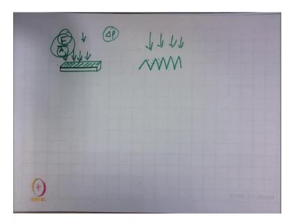
In flat filter, the shape is in flat condition, when air is flowing. Here the area of the filter surface area of the filter is limited that is why, the pressure drop will be more pressure drop is of that is force by unit area. Now, if we can somehow increase the area by having same force value, we can reduce the pressure drop, this is done by making pleats. This is
