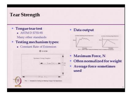
After tensile strength, the tear strength is also important which is tongue tear strength, where this is a specimen of dimension 200 millimeter by 75 millimeter as per ASTM standard. And the cut is made of 75 millimeter length, and this two sides are gripped with the jaws of a tensile tester, and tensile test is carried out. And the fabrics will tear through this zone.
