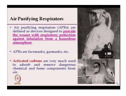
Next is that air purifying respirators, which is used as facemask ok. Air purifying respirators are defined as the devices designed to provide the wearer with respiratory protection against inhalation from hazardous atmosphere. APRs are facemasks, gasmasks, etcetera. Activated carbons are also used to absorb and remove dangerous chemicals and fumes.
