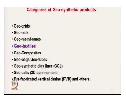
So, if we try to categorise the geosynthetics; that means, geosynthetics are the material which are used for civil engineering construction related to soil or related to any other construction. So, this geosynthetic products can be categorised in terms of geo grids, geo nets, geo membranes, geotextiles the part which we will cover here, geocomposites, geobag or geotubes, geo synthetic clay liner, geocell which is 3 dimensional confinement
