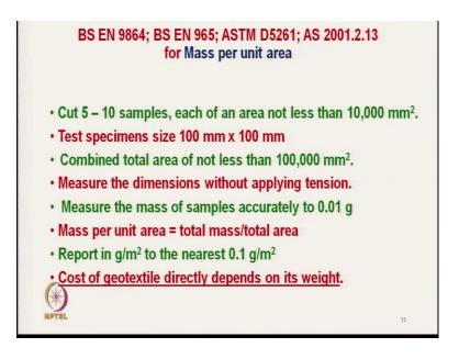
Next characteristics is mass per unit area; we can test mass per unit area by many standards like BS EN 9864, BS EN 965 ASTM D 5261 ASTM 2001.2.13 any method we can use and this methods if you follow, we can get the mass per unit area of geotextiles. So, here what we have to do we have to cut typically 5 to 10 samples each of having area not less than 10000 square millimetre; that means, if you want to get the sample specimen.
