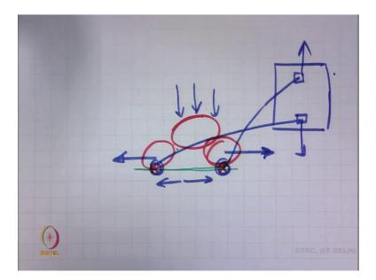
Here now let us discuss here this is geotextile and we have say stones and these are the contact points, gripping points we can say. Now when load is applied vertically, this stones will try to move sideways. Having this two points gripping point the geotextile
