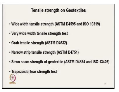
So, there are different types of tensile strengths, first is wide width tensile strength its as per ASTM D 4595 and ISO 10319, then very wide width tensile strength next is grab tensile strength as per ASTM D 4632, then narrow strip tensile strength which is as per ASTM D 4751, third sewn seam strength of geotextile this is actually tensile strength, but in the seam portion because geotextile when we are laying we must incorporate stitches.
