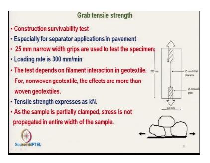
Next characteristics says that, grab tensile test. So, this is construction survivability test. Its not only the tensile test this test will give idea about the survivability of the structure how the structure will survive during application of load for long time specially for separator applications in pavement.
