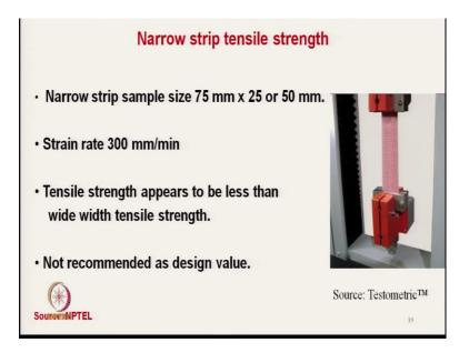
We sometime test the geotextile in narrow strip tensile mode also, but size of the strip is 75 mm by 25 mm strain rate is 300 mm/minute tensile strength appear to be less than the wide width tensile strength here. And this test its for index testing only, its not recommended for design value. So, the value we cannot use for designing the geotextiles for using in any project.
