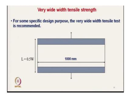
In some application we may need very wide width tensile strength. So, where the width of the specimen is as high as 1 meter width. So, we have to design the jaw accordingly and the length is half of that. So, half metre, 1 meter by half metre its the actual test specimen size.
