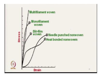
So, if we see the comparative stress strain curves for different types of geotextiles, here its a monofilament woven fabric and next one is multifilament woven fabric. So, monofilament woven fabric although the breaking stress is less than the multifilament woven fabric, but the monofilament woven fabric has got higher modulus. Multifilament woven fabric has relatively lesser modulus than monofilament, but this multifilament woven fabric has got very high tensile strength.
