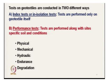
So, there are two different types of test which are conducted on geotextiles. One is called index testing or in isolation test, which actually test in the laboratory condition. So, only the tests are performed on geotextile next is that its called performance test what is that? The performance test are performed along with site specified soil and conditions.
