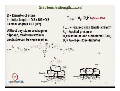
Now, let us see the analysis here D is the average diameter of stone, 1 1 is the initial grip length this is the initial grip length here. Now assumption here is that they are the stones are spreaded equal equidistant.
