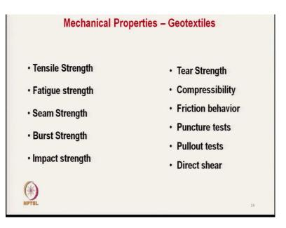
In mechanical properties there are tensile strength, fatigue strength, seam strength, bursting strength, impact strength, tear strength, compressibility of geotextiles, frictional behaviour of geotextiles, puncture tests, pullout test and direct shear test. So, we will discuss all these test methods one by one first let us start with the measurement of tensile strength.
