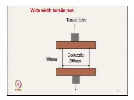
This is the schematic diagram where width of the geotextile is 200 mm and length of the specimen is 100 mm, actual specimen length will be more than this, but gauge initial gauge length is 100 mm. So, due to this wide width the Poisson's ratio is restricted and this value the result which we get here from wide width tensile test it simulates the actual field condition.
