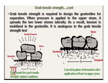
Now, let us try to see the analysis. A grab tensile strength is required to design the geotextile for separation. So, this is for separation purpose here when pressure is applied to the upper stone. So, when its applied it spreads the 2 lower stone laterally.
