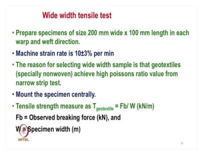
First we will discuss the wide width tensile test, where you must prepare a specimen of size 200 millimeter wide, so, 20 centimetre wide and 10 centimeter length in each warp and weft direction.
