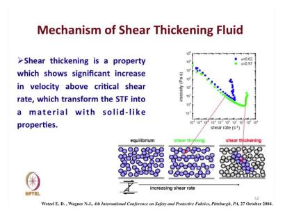
Now, if you see the mechanism of shear thickening fluid is that the shear thickening is a property which shows significant increase in velocity above critical sorry viscosity so this is the viscosity. So, shear thickening is that as we increase the shear rate shear thickening fluid will result significant increase in viscosity above a critical shear rate. So, this is the critical shear rate which transforms the shear thickening fluid into a material which is definitely solid like.
