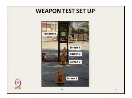
So, this is a test system where this is screen 1, screen 2, screen 3, and screen 4 are there and this is the fabric specimen. So, we can if we measure the speed between this before striking and after striking we can calculate the energy absorbed.
