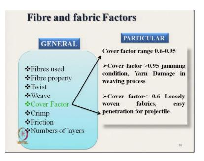
Cover factor is extremely important characteristics. So, it should range between 0.6 to 0.95, that is the range it should not be too high. If it is more than 0.95 then the jamming condition will be created and that will result yarn damage during weaving process and if yarn damages takes place during weaving.
