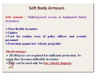
So, these are basically multilayered woven or laminated fabric structure. Typically they are supposed to be flexible and lighter in weight. So, they are relatively more flexible in nature than hard body armour lighter in mass. And they are used for routine wear of police officers and security personnel. The soft body armours normally do not use for high threat zone. So, they are providing protection against low velocity projectiles.
