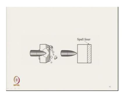
In hard body armours the deformation if it penetrates and the particles this particles will be coming out from the other side. That is why spall liner is provided so that it stops these particles to come out from the structure.
