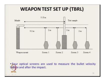
Another test is that weapon test setup, this is weapon test where there are different screens. Screen 1, screen 2, screen 3, screen 4 these are the different screen. So, four optical screens are used to measure the bullet velocity before and after the impact. So, different screens are used. So, we need to calculate the difference in speed for that we have to measure the speed of bullet before striking the fabric and the speed after it is penetrating through the fabric.
