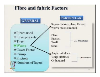
Then comes weave structure; so the structure of fabric, it should be square fabric plain structure or basket weave are most common. So, plain basket they are most commonly used with the square structure. And twill or satin sometime is being used all these structures are two dimensional structures in addition to two dimensional structure sometime we use 3D structures. Like angle interlock warp interlock orthogonal to enhance the impact performance of the clothing.
