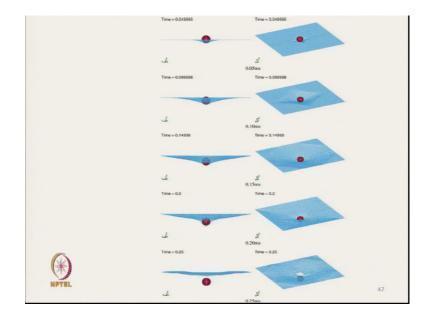
So, these are the schematic representation. So, gradually the impactor is impacting on the material and deflection is taking place. But if the velocity is very high it may sometime penetrate through the structure this is the only one layer we are talking about.
