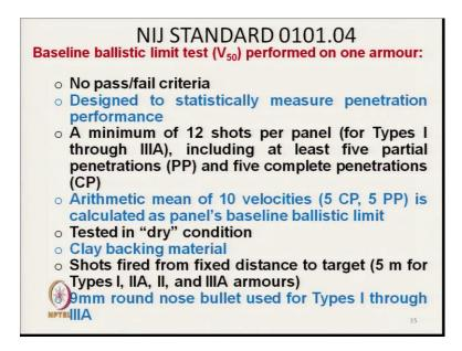
And as far as NIJ standard 0101.04, Ballistic baseline ballistic limit which is said as  $V_{50}$  which is performed on one armour. So, the method is here no pass fail criteria is decided only the velocity, which we try to find where the probability of penetration is 50 percent that is denoted as  $V_{50}$ . So, designed to statistically measure the penetration performance.
