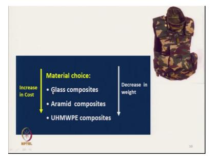
So, as the developments are going on the materials requirement towards decrease in weight we need lighter ballistic protective clothing at the same time the cost is increasing. So, materials choice are also changing initially we use the glass composite then aramid composite and then ultra high module molecular weight polyethylene composite.
