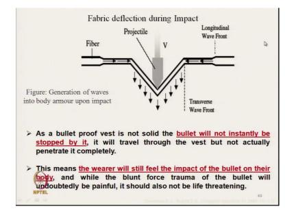
So, as we have seen that this will create and wave and that speed of this wave depends on the properties of fibre. So, as a bullet proof vest is not solid the bullet will not instantaneously be stopped. So, it will not be stopped instantly rather it will travel through the vest, but not actually penetrate it completely ok.
