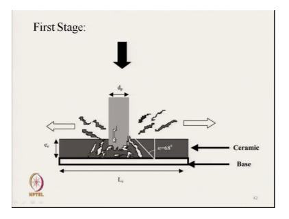
So, this is the first stage; once it is striking the particles are coming out this is a ceramic hard body armour and this is the base and after certain time.
