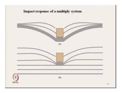
So, this is the type of representation first layer second layer third layer so there are different layers. So, it is penetrating through one layer, then second layer after second time there will be accumulation of layers next layers. So, it will ultimately stop in between this structures.
