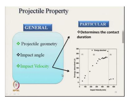
So, as the impact velocity is increasing here in the x axis it showing the impact velocity y axis it is showing the energy absorbed. As the impact velocity increases so initially the energy absorption will increase.
