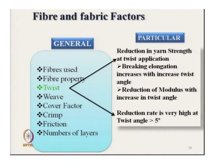
After the fibre property then yarn twist is a also very important reduction in yarn strength occurs when we apply twist that is very well known fact. And also with the increase in twist angle the breaking elongation also increases. So, we have to create yarn structure which has got high strength and low breaking elongation.
