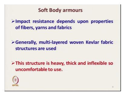
So, in soft body armours the impact resistance that is protection depends on the properties of fibres yarns and fabrics. So, we will see how fibres yarns and fabrics affect the impact resistance of soft body armours.
