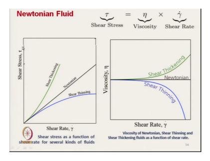
So, this curve shows that shear rate in the x axis shear stress in the y axis. For a Newtonian fluid the shear stress and shear strain they are proportional ok. So, that we will have constants so straight line. So, this is the value viscosity remains constant so for Newtonian fluid. But for non Newtonian fluid the viscosity may increase with the increase in shear rate or may decrease with the increase in shear rate.
