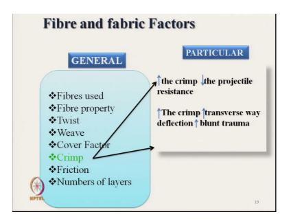
Next is crimp; which is very important for ballistic protective clothing we should have fabric with least crimp in yarn. So, if we increase the crimp so projectile resistance will be reduced. So, as the crimp increases transverse way deflection will increase which will result blunt trauma. This blunt trauma measurement process I will discuss later in this class.
