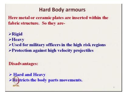
The hard body armour are those where metals and ceramic plates are inserted within the structure. So, due to this metal and ceramic insertion they are becoming rigid, they are heavy. And all this hard body armours are used for military officers in the high risk region because this hard body armours are meant for the high threat.
