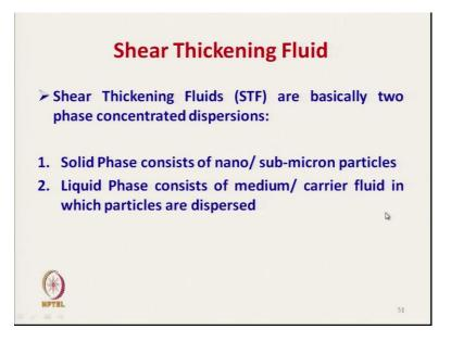
So, first you must understand what is shear thickening fluid. These are basically two phase concentrated dispersions. Phase 1; which is solid phase which consists of nano or submicron particle. And phase 2; is that liquid phase which consists of a medium or carrier fluid which carries the particles in dispersed condition.
