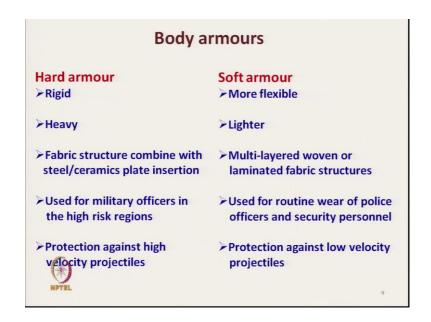
So, if you see broadly the difference between hard body armour and short soft body armours. The hard body armours are rigid whereas, soft body armour are relatively flexible. Hard body armours are heavy this soft body armours are lighter. Fabric structure combined with steel or ceramic plates insertion. Whereas, in case of soft body armour we do not need any insertion, but here multilayered woven or laminated fabric structures are used.
