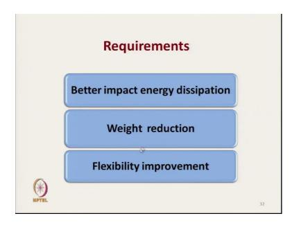
So, the requirements are in short better impact energy dissipation. So, the ballistic protective clothing should be able to dissipate the energy in a better way. The mass should be lower so weight reduction should be there and it should be flexible. So, that proper handle, proper comfort characteristics should be there.
