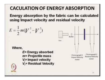
So, this is the energy absorption by fabric can be calculated using impact velocity and residual velocity. So, these are the different sensors here. So, energy absorbed E equal
