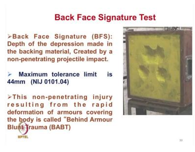
So, this is the back face so and the depth we can measure ok. Back face signature it is a depth of the depression made in the backing material. This yellow colour this is the backing material created by non perforating projectile impact ok. Maximum tolerance limit is 44 millimeter as per NIJ standards, this maximum depth should be 44 millimeter.
