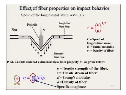
So, the fabric which we are making from a fibre with different characteristics that will affect the impact behaviour. So, effect of fibre properties on impact behaviour. This diagram shows here projectile is striking on the surface of the fabric and that will result the longitudinal wave. And the speed of this wave the longitudinal wave in the side way that way is expressed in terms of initial modulus of fibre and density of fibre which means that C equal to
