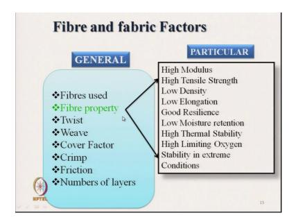
Like in fibre properties the fibre should have high modulus ok. Then high tensile strength low density because we need mass should be low it should be lighter low elongation if it elongates if it is elongation is very high then the impact performance impact resistance will be affected. Good resilience it should come back from the deformation. Low moisture retention so if the fibre retains moisture, then it is mechanical behaviour may get affected.
