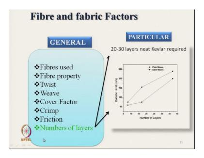
So, it is obvious if we increase the number of layer the ballistic limit will increase energy absorption will increase. But at the same time the mass of the total structure will increase which will result uncomfortable sensation.
