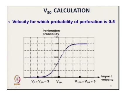
So, this is the velocity probability curve. So, as the velocity increases so where velocity say 0 so there is no penetration. And as we increase the velocity, the probability of penetration increases and when the velocity is say  $V_{100}$  at that velocity there will be 100 percent penetration.
