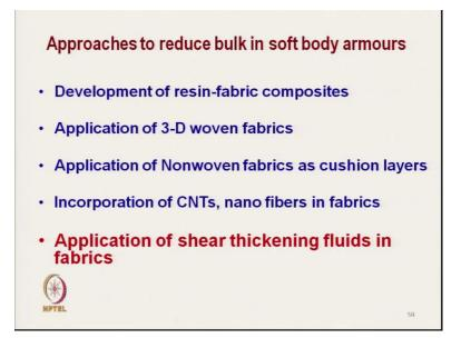
So, approaches to reduce the bulk in soft body armours. So, we have seen that in soft body armour we can use a number of layers say 30 40 layers that will effectively increase the bulk of the body armour. So, there are different approaches which reduces the bulk. These are development of resin fabric composites, application of 3-D woven fabrics, application of non woven fabrics as cushion layers.
