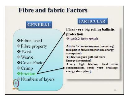
Next important characteristics is friction. Friction is also very important characteristics and typically the frictional coefficient of 0.2 is a optimum value. As the frictional coefficient increases the basic thing what happens due to increase in friction between yarn more and more secondary yarn will come into picture due to frictional contact. And those yarns will take part in the resistance and absorption of energy.
