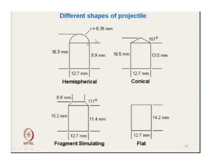
So, these are the different shapes hemispherical tip, conical tip, fragmented tip, and flat tip different types of shapes.
