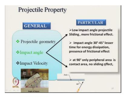
Then impact angle is also important low impact angle properties actually this is the angle with the surface and this is the projectile. So, low impact angle projectile it affect the sliding and more frictional effect. So, it if the angle is low the projectile instead of penetration it will slide
