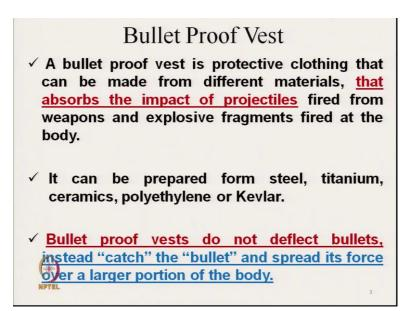
So, bulletproof vest which is coming under ballistic protective textiles is a protective clothing that can be made from different material which absorbs the impact of projectiles that is a bullet fire from weapons and explosive fragments fired at the body. So, this bulletproof vest has to protect us from all this impacts. So, this vests can be prepared from steel, titanium, ceramics, polyethylene or Kevlar.
