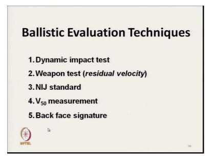
There are different methods so ballistic evaluation techniques are dynamic impact test weapon test which actually measures the residual velocity. So, after penetration what is the velocity remaining in the projectile that we measure.
