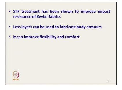
So, shear thickening fluid treatment has been shown to improve impact resistance of Kevlar fabric. So, if we use shear thickening fluid we can get effective characteristics with less number of layers. It can improve flexibility and comfort characteristics as we use less number of fabric layers.
