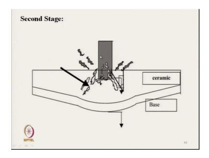
Next stage this is the state where the base will have deformation and there will be particles.
