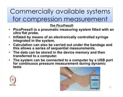
Another commercially available system is it is a PicoPress, it is a pneumatic measuring system fitted with ultra flat probe. So, here its ultra flat probes are there which is pneumatic
