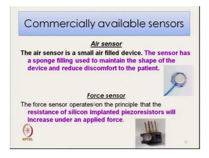
There are other methods like air sensor, it is a small air filled device. The sensor has a sponge field used to maintain the this sponge filling it is to maintain the comfort level of the patient. Force sensor can also be used here.
