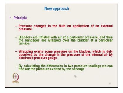
Now, the principle of the new instruments is that pressure changes in the fluid on application of external pressure that is the basic principle. Suppose, we inject some air in
