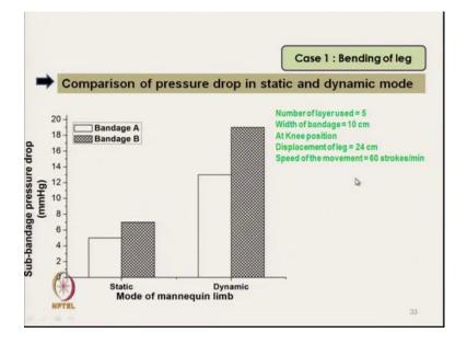
And this picture shown, this figure showing the sub bandage pressure with a static mode and the dynamic mode, this is the drop in pressure. So, if you see in static mode both for bandage A and B, the pressure drop is least so, which is required, but once the person is dynamic, the pressure drop is much higher than that; the which means, after putting bandage a person if he moves, the pressure drop will be high; that means, reduction in pressure of compression bandage will be high.
