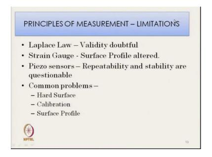
So, principles are there ok, different principles of measurements are there. So, Laplace law we can use the Laplace law principle, but the limitations are so validity is doubtful ok. We can use strain gauge principle for measurement of compression pressure, but there we cannot have smooth surface like our limb our body part, the surface profile has to alter, then we can use the strain gauge.
