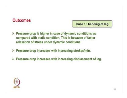
So, the outcome of case 1 is that, pressure drop is high in case of dynamic condition as compared with the static condition. This is because of faster relaxation of stress under dynamic condition, pressure drop increases with the increase in stroke per minute and pressure drop increases with increasing displacement of leg.
