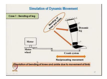
Now, this is one equipment, the schematic diagram of the equipment here as we have discussed we will consider here two situations; one is bending of leg, so, this is the leg mannequin and motor, it is attached with the motor and the bending level and the rate of stroke can be changed.
