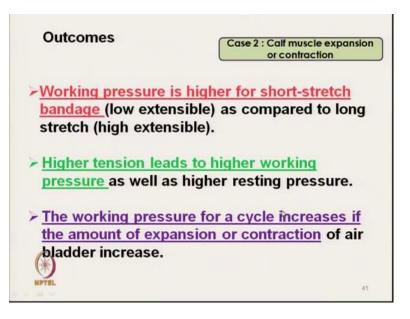
And this we have discussed here and the outcome here, the result here, the working pressure is higher for short-stretch bandage, that we have used two types of bandage, short-stretch bandage and long-stretch bandage. Short-stretch bandage is low extensible bandage and long stretch bandage is highly extensible bandage so, pressure is high if we can develop a short stretch bandage.
