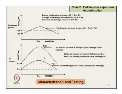
So, this result it shows the with time that is the cycle time is 30 second, this is 30 second cycle time; as we increase this is air bladder pressure one cycle without bandage as we increase the pressure; the calf muscle expansion, its simulating the calf muscle expansion, the air pressure is increased and then it is decrease.
