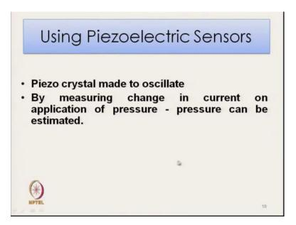
Another method which is piezo crystal based method; piezo electric sensors are used and piezo crystals are made to oscillate by measuring the change in current on application of pressure, pressure can be estimated.
