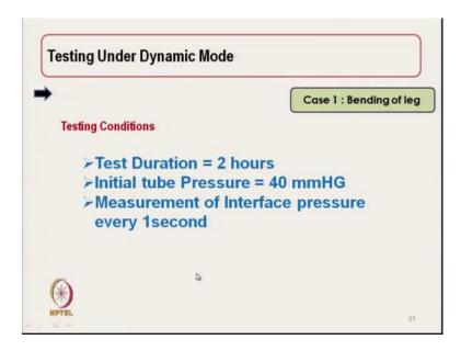
And test duration is 2 hour, initial pressure is 40 millimetre HG, initial pressure actually shows the limb hardness, measurement of interface pressure is done after every 1 second and this is the result here.
