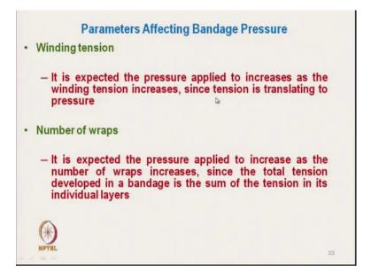
And the parameters which has already been discussed, this parameters are winding tension, number of wraps, width of the bandage, time elapsed after bandaging.
