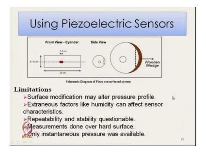
So, here the limitations are same as that we have discussed earlier. Surface modification is required which may alter the pressure profile, external factors are the affecting factors like humidity temperature, repeatability and stability is questionable, measurements done over hard surface and here one most important limitation only instantaneous pressure was available so, continuous pressure profiling is a problem.
