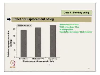
Here this picture shows that, the displacement of mannequin limb as the displacement increases from 12 centimetre to 24 centimetre, the pressure drop increases; that means, if the bending of the limb, bend is there it is more or if the step length is more, if he is walking
