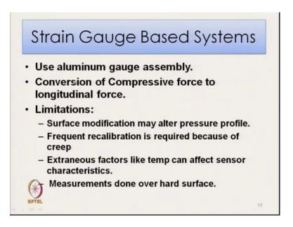
Next principle of measurement of compression bandage is strain gauge based principle where aluminium gauge assembly is used and the conversion of compressive force to longitudinal force is required and the limitation is that the surface modification may alter the pressure profile. So, we need surface modification because we have to place the strain gauge on the surface and that total profile of the bandage also changes which also alter pressure profile.
