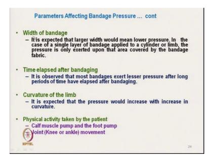
This is one important parameter because, when we start recording the pressure just after bandaging, the pressure is high, but as the time elapsed after bandaging. It is observed that most bandages exert less lesser pressure after long period due to creep effective stress.
