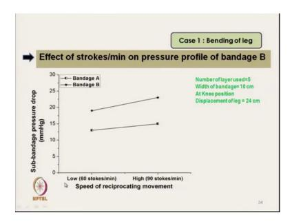
This figure shows the speed of reciprocating movement. Once, the person moves at slower speed the pressure drop is less, but with the increase in speed the pressure drop is high, this is due to structural change of the bandage.
