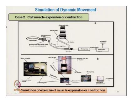
And in case 2, where the calf muscle expansion or contraction have been reported like this is, these are the different diameters of calf muscles and the black colour these are the bladders which are inflated by using pump and this pump are inflated and deflated cyclically to simulate the calf muscle expansion. And over this bladder the compression bandage is wrapped.
