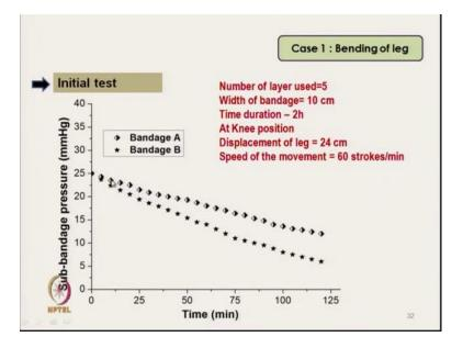
Which shows the sub bandage pressure, it reduces as time elapse with the time sub bandage pressure reduces gradually; that means, there is stress relaxation for both bandage A and bandage B, but the ideal bandage should be that there should not be reduction in sub
